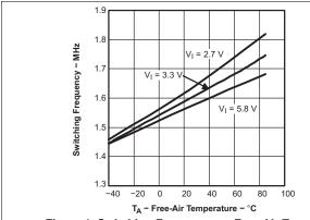
Figure 1. Switching Frequency vs Free-Air Temperature
