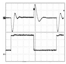
Figure 9. Overcompensated (Damped Oscillation),  $R_{\rm C}$  is Too Large
