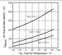
Figure 2. r<sub>DS(on)</sub> N-Channel Main Switch vs Free-Air Temperature
