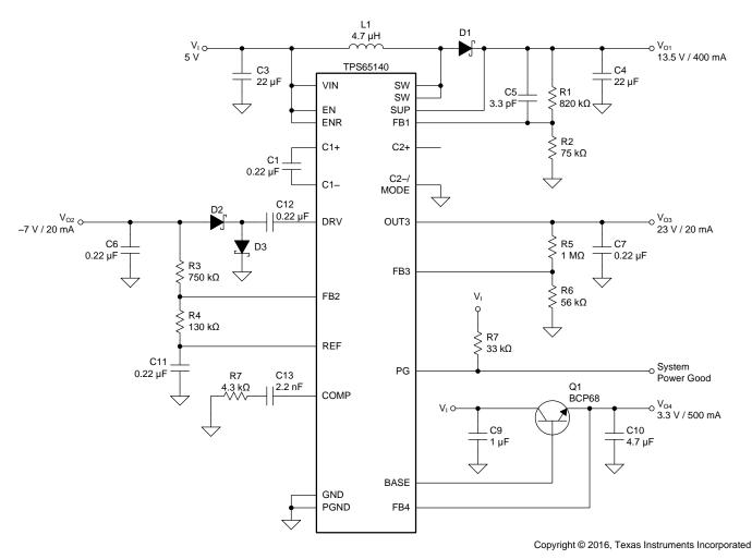
Figure 25. Typical Application, Monitor Supply
