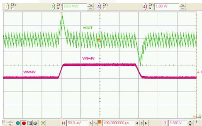
Figure 20. Line Transient, 50\ \Omega Load, t_R=t_F=10\ \mu\text{s}
