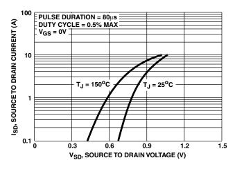
FIGURE 13. SOURCE TO DRAIN DIODE VOLTAGE
