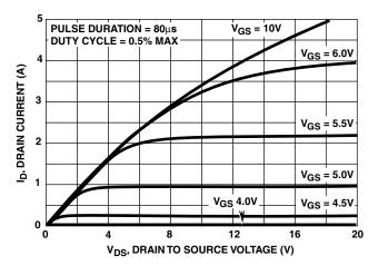
FIGURE 6. SATURATION CHARACTERISTICS
