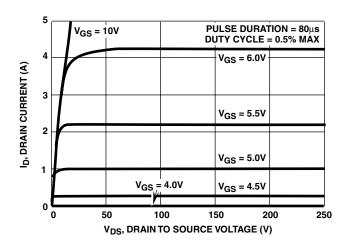
FIGURE 5. OUTPUT CHARACTERISTICS
