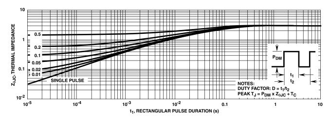
FIGURE 3. MAXIMUM TRANSIENT THERMAL IMPEDANCE
