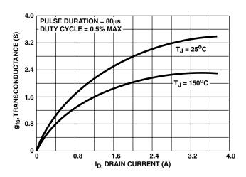
FIGURE 12. TRANSCONDUCTANCE vs DRAIN CURRENT
