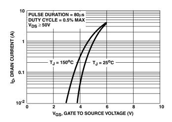
FIGURE 7. TRANSFER CHARACTERISTICS
