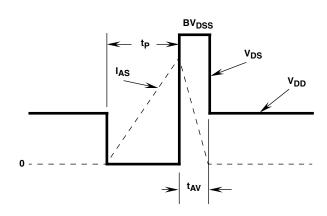
FIGURE 16. UNCLAMPED ENERGY WAVEFORMS
