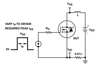
FIGURE 15. UNCLAMPED ENERGY TEST CIRCUIT
