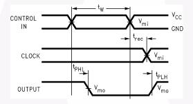
Propagation Delay. Pulse Width and  $t_{rec}$  Waveforms
