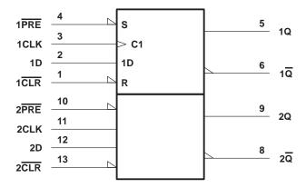
$<sup>\</sup>dagger$  This symbol is in accordance with ANSI/IEEE Std 91-1984 and IEC Publication 617-12. Pin numbers shown are for the D, DB, DGV, J, NS, PW, and W packages.
