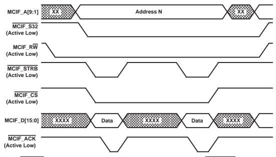
NOTE: MCIF\_CS can be deasserted between the data phases of a 32-bit access. The MCIF\_STRB signal acts as the master enable for MCIF.
