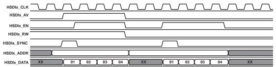
Figure 3–24. Functional Timing for Multistream Mode (Read and Write)
