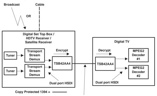
The set box sends multiple PES packets to the digital TV on either one transport stream on one Iso channel OR on two different transport streams on two different Iso channels.
