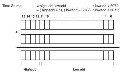
Figure 4–6. Determination of Highadd and Lowadd
