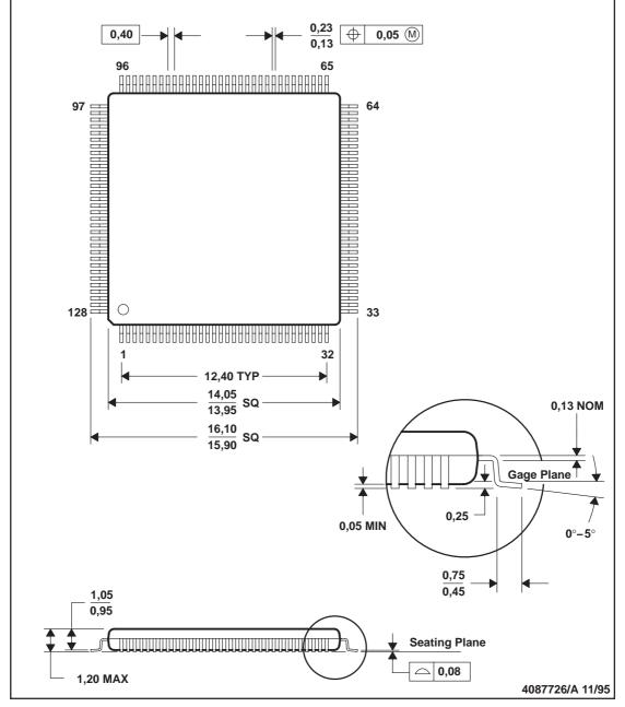
NOTES: A. All linear dimensions are in millimeters. B. This drawing is subject to change without notice.
