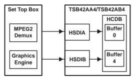
Figure 3–14. *HSDI* Single-Stream Mode Example
