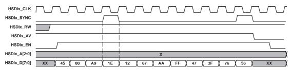
Figure 3–17. HSDI Read, Byte Wide Data Bus, Sync Mode C
