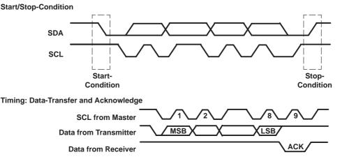
Figure 3–26. Two-Wire Serial Interface Bus Protocol
