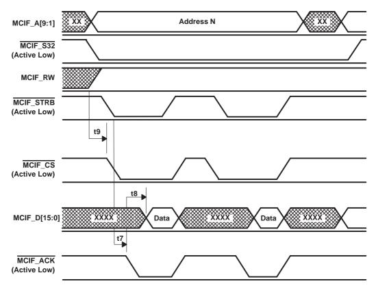
Figure 3–7. Microcontroller Interface Critical Read Timing
