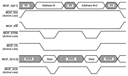
NOTE: MCIF\_CS can be deasserted between the two 16-bit transactions. The MCIF\_STRB signal acts as the master enable for MCIF.
