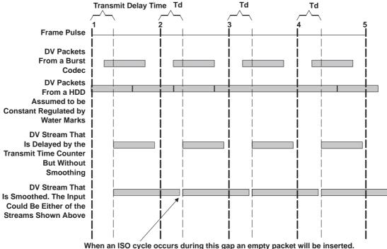
It is possible for up to two empty packets to occur during this gap.
