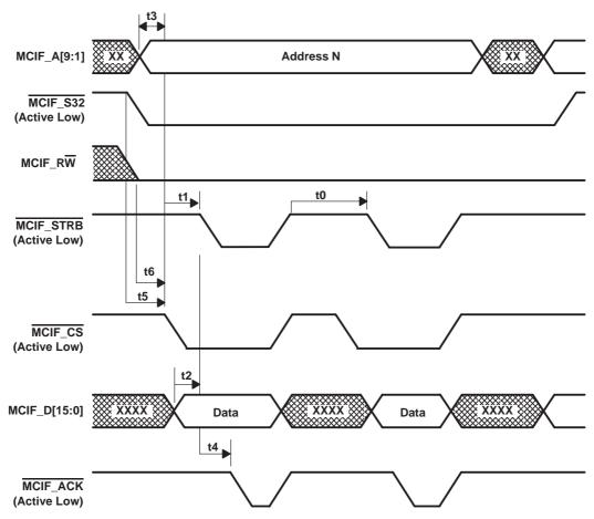
Figure 3–6. Microcontroller Interface Critical Write Timing
