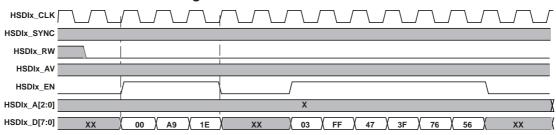
Figure 3–19. HSDI Write, Byte-Wide Data Bus, Sync Mode A
