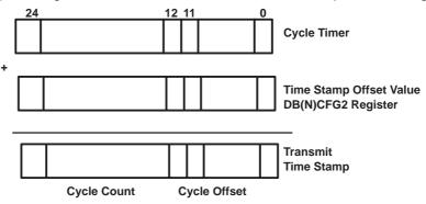
Figure 4–4. Determination of Transmit Time Stamp
