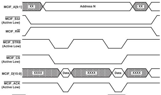
NOTE: MCIF\_CS can be deasserted between data phases of 32-bit read. The MCIF\_STRB acts as the master enable for the MCIF.
