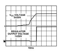
Figure 11. Power-On Start-Up Waveforms
