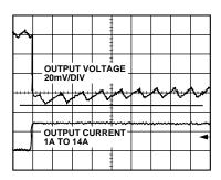
Figure 10. Transient Response, 1A–14 A of Figure 2 Circuit
