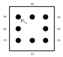
Figure 2. 8-Bump DSBGA Top View
