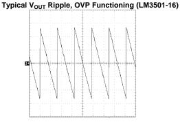
$V_{OUT}$  open circuit and equals approximately 15V DC,  $V_{IN} = 3.0V$ 3)  $V_{OUT}$ , 200 mV/div, AC
