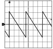
$V_{OUT}$  open circuit and equals approximately 20V DC,  $V_{IN} = 3.0V$ 1) V<sub>OUT</sub>, 200 mV/div, AC
