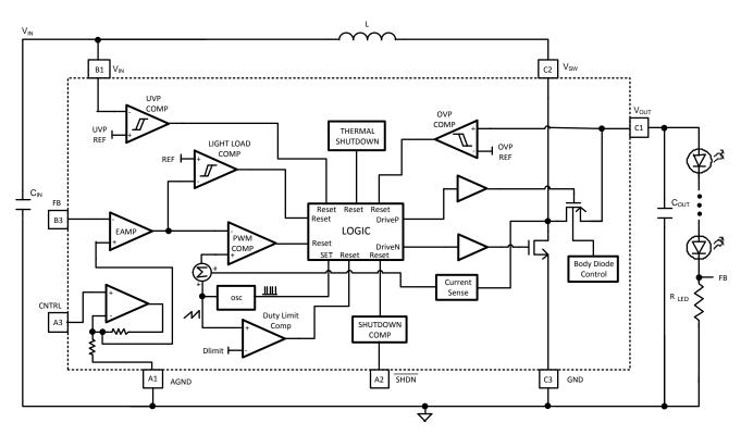
Figure 33. LM3501 Block Diagram
