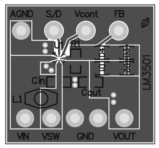
Figure 34. Evaluation Board Layout (2X Magnification)
