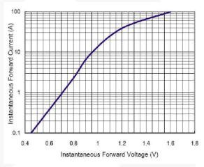
Figure 4. Typical Forward Characteristics per Leg
