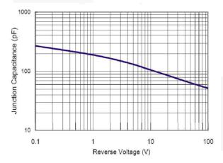
Figure 5. Typical Junction Capacitance
