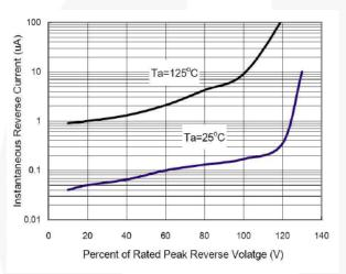
Figure 3. Typical Reverse Characteristics per Leg
