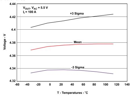
Figure 1. Typical OUT Voltage Regulation, bq24032A
