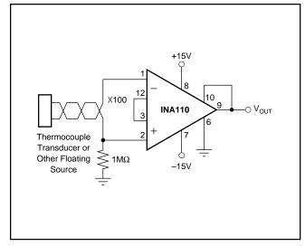
FIGURE 7. Floating Source Instrumentation Amplifier.
