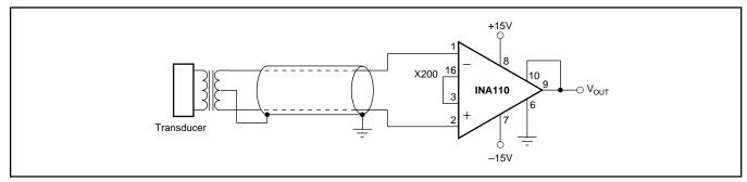
FIGURE 6. Transformer-Coupled Amplifier.
