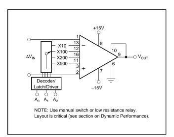
FIGURE 11. Programmable-Gain Instrumentation Amplifier (Precision Noninverting or Inverting Buffer with Gain).
