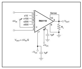
FIGURE 1. Basic Circuit Connection.
