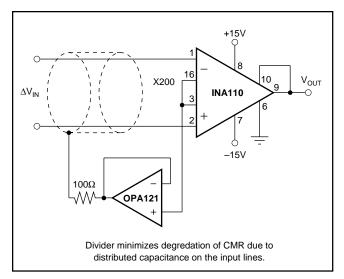
FIGURE 8. Instrumentation Amplifier with Shield Driver.
