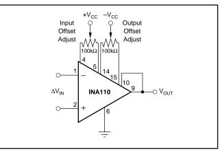
FIGURE 2. Offset Adjustment Circuit.
