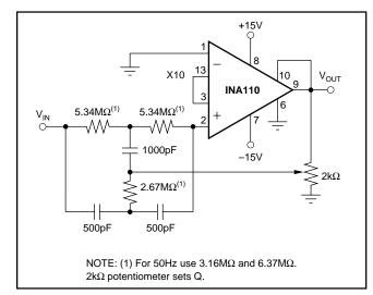
FIGURE 13. 60Hz Input Notch Filter.
