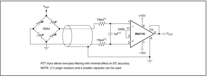
FIGURE 9. Bridge Amplifier with 1Hz Low-Pass Input Filter.
