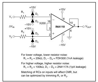
FIGURE 14. Input-Protected Instrumentation Amplifier.
