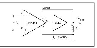
FIGURE 5. Current Boosting the Output.
