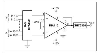
FIGURE 12. Rapid-Scanning-Rate Data Acquisition Channel with 5µs Settling to 0.01%.
