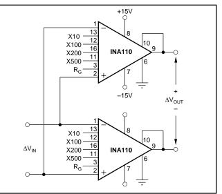
FIGURE 18. Differential Input/Differential Output Amplifier.
