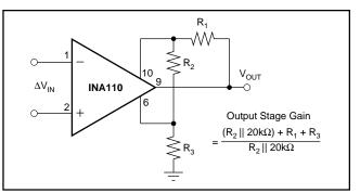
FIGURE 4. Gain Adjustment of Output Stage Using H Pad Attenuator.
