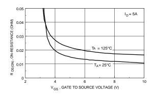
Figure 4 . On Resistance Variation with Gate-to-Source Voltage.
