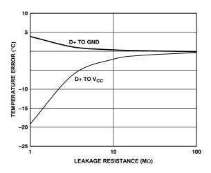
Figure 6. Temperature Error vs. D+/D- Leakage Resistance
