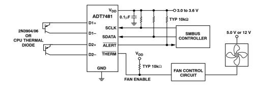
Figure 22. Typical Application Circuit
