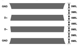
Figure 21. Typical Arrangement of Signal Tracks
