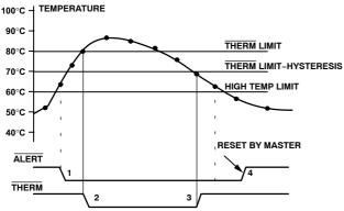
Figure 19. Operation of the ALERT and THERM Interrupts
