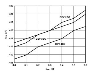
Figure 9. Operating Supply Current vs. Voltage
