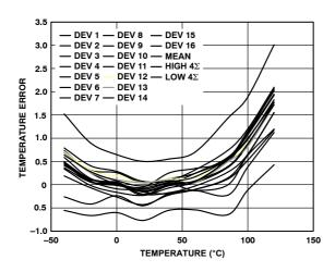
Figure 3. Local Temperature Error vs. Temperature
