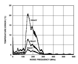
Figure 12. Temperature Error vs. Common-Mode Noise Frequency
