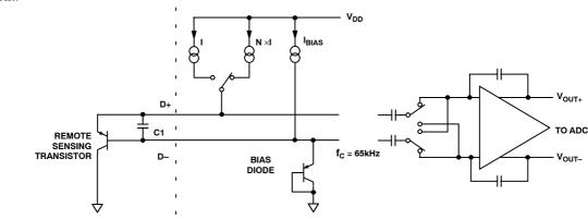
Figure 14. Input Signal Conditioning
