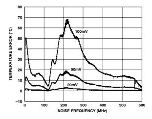
Figure 13. Temperature Error vs. Differential Mode Noise Frequency
