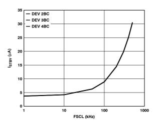
Figure 11. Standby Supply Current vs. SCLK Frequency
