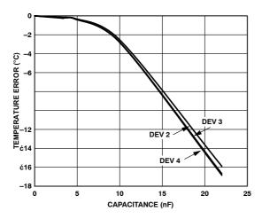
Figure 7. Temperature Error vs. D+/D- Capacitance
