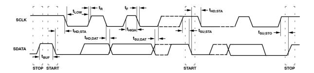
Figure 2. Serial Bus Timing
