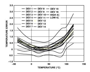
Figure 4. Remote 1 Temperature Error vs.
