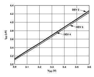
Figure 10. Standby Supply Current vs. Voltage
