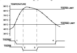
Figure 20. Operation of the THERM and THERM2
