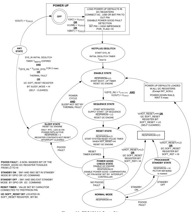
Figure 28. TPS65820 State Diagram
