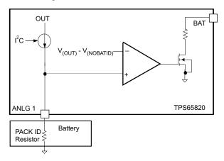
Figure 33. Battery Removal Detection, ANLG1 Pin
