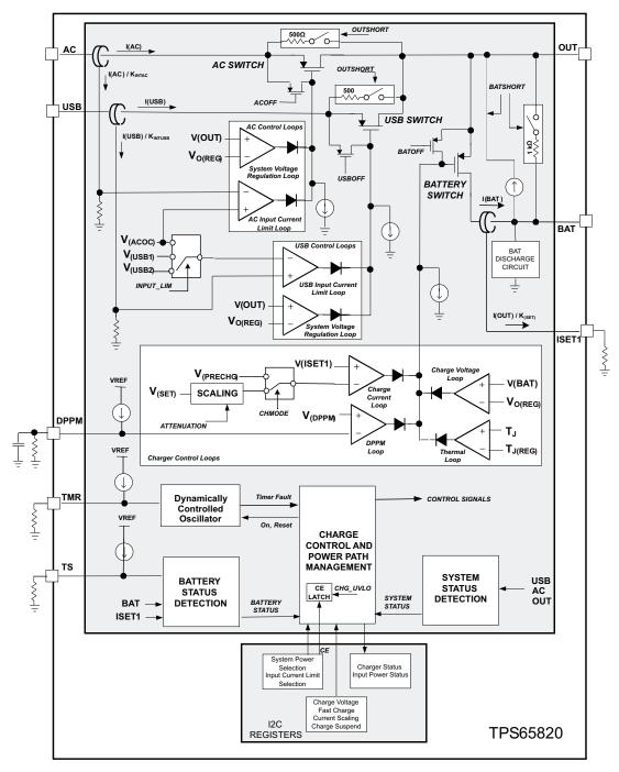
Figure 31. TPS65820 Charger and Power Path Section Simplified Block Diagram
