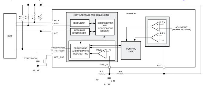
Figure 27. Simplified Block Diagram
