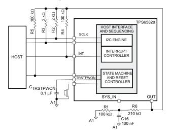
Figure 26. Required External Components, Recommended Values, External Connections
