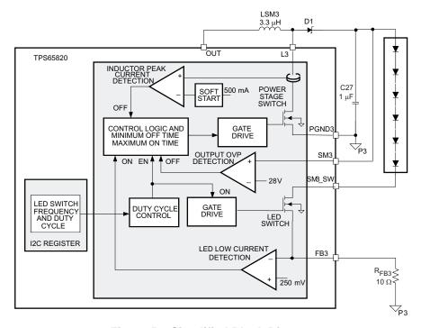
Figure 54. Simplified Block Diagram
