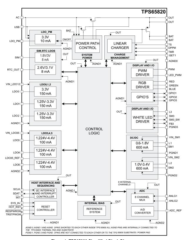
Figure 1. TPS65820 Simplified Block Diagram
