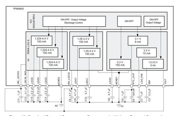
Figure 39. Required External Components, Recommended Values, External Connections
