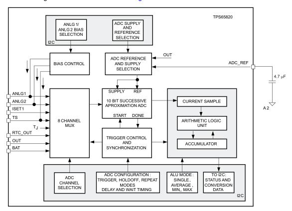
Figure 48. ADC Simplified Block Diagram
