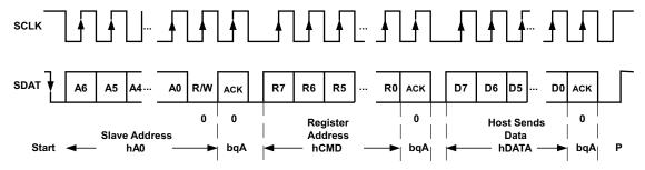
Figure 25. I<sup>2</sup>C read and write operations
