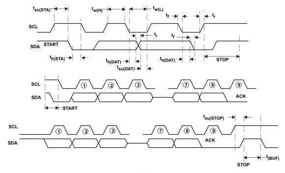
Figure 2. I<sup>2</sup>C Timing
