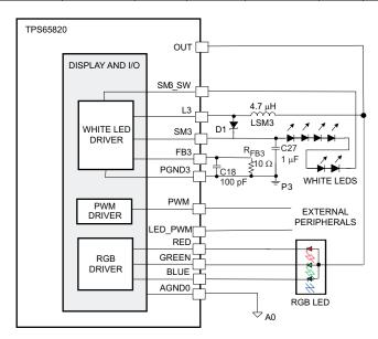
Figure 53. Required External Components, Recommended Values, External Connections
