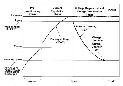
Figure 34. Typical Charge Cycle, Thermal Loop not Active
