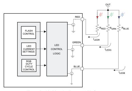
Figure 57. Limiting the External LED Current
