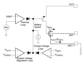
Figure 35. Voltage and Thermal Regulation Loops
