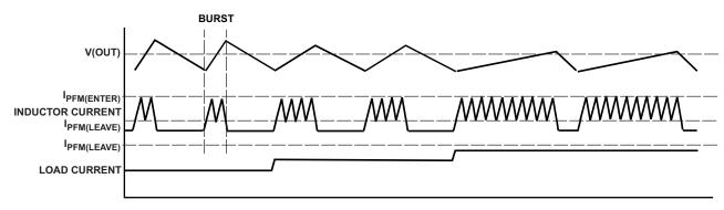
Figure 46. Typical Burst Operation in PFM Mode
