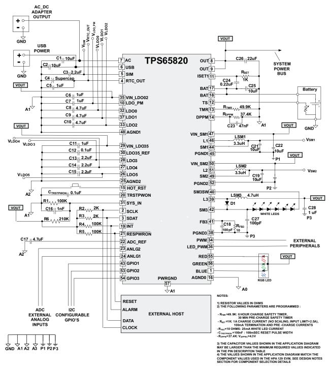
Figure 3. TPS65820 Application Diagram, Recommended External Components
