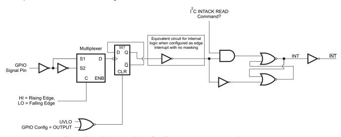
Figure 59. GPIO 1 or GPIO2 Configured as an Interrupt Request Input
