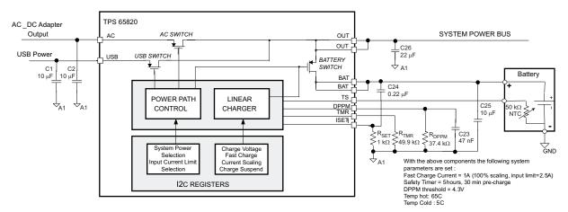
Figure 30. Required External Components, Recommended Values, External Connections
