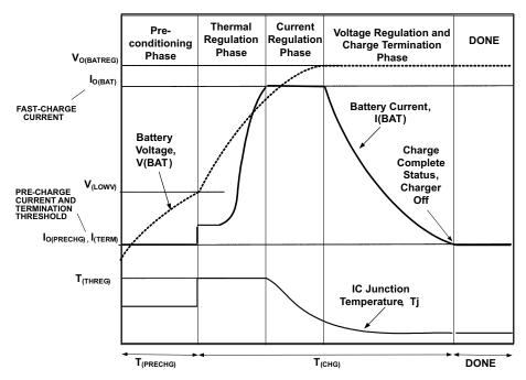
Figure 36. Typical Charge Cycle, Thermal Loop Active
