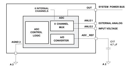
Figure 47. Required External Components, Recommended Values, External Connections
