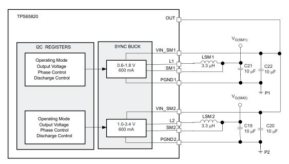
Figure 41. Required External Components, Recommended Values, External Connections
