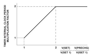
Figure 38. Safety Timer Internal Clock Slowdown
