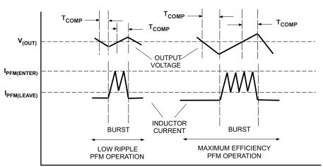
Figure 45. PFM mode operation waveforms
