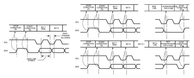
Figure 24. I<sup>2</sup>C operation waveforms
