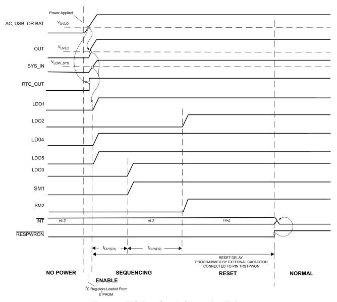
Figure 29. TPS65820 Supply Sequencing Timing
