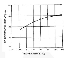
Figure 3. Adjustment Current
