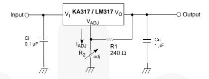
$$V_0 = 1.25 \text{ V} (1 + R_2 / R_1) + I_{ADJ}R_2$$
