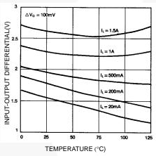
Figure 4. Dropout Voltage
