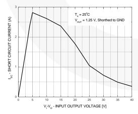
Figure 6. Short Circuit vs. Input-Output Voltage
