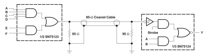
Figure 3. Unbalanced Line Communication Using SN75123 and SN75124
