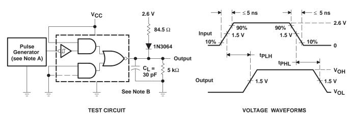
NOTES: A. The pulse generator has the following characteristics:  $Z_O \approx 50~\Omega$ , PRR  $\leq 5~MHz$ , duty cycle = 50%.
