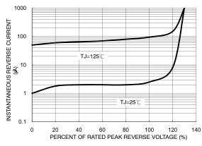
Figure 2. Typical Reverse Characteristics
