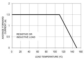
Figure 1. Forward Current Derating Curve
