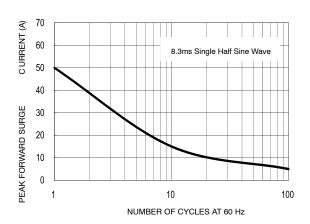
Figure 3. Maximum Non-Repetitive Forward Surge Current
