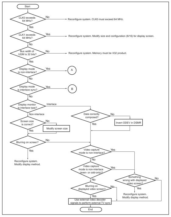
Figure J.4 Q2SD Video Setting Flow (1)
