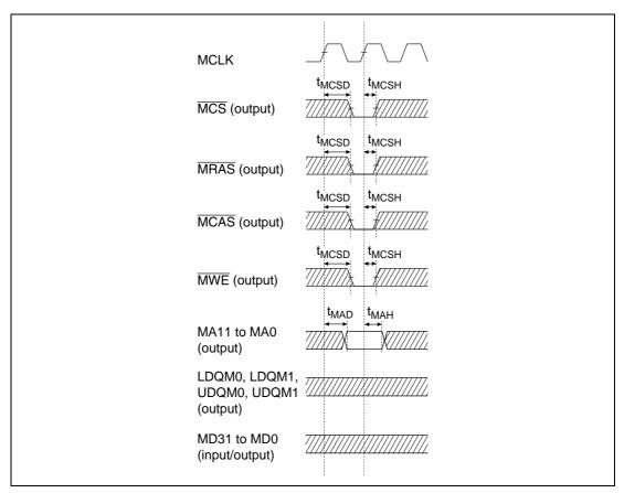
Figure 7.11 (2) UGM Mode Register Setting Cycle Timing
