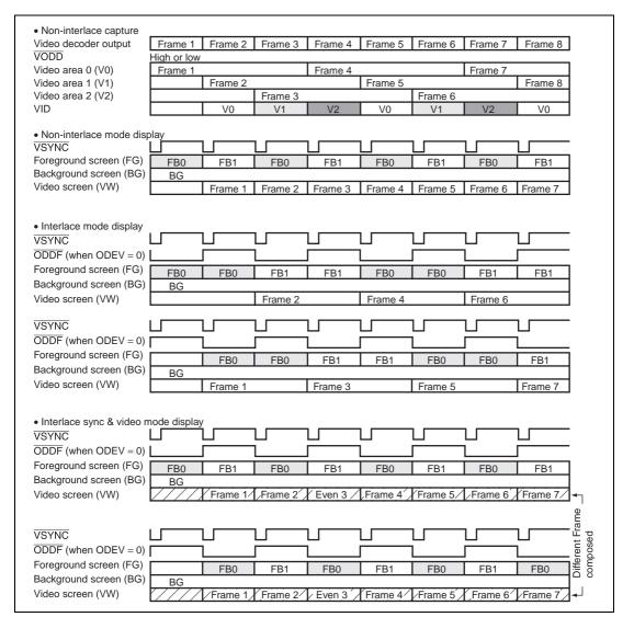
Figure 3.70 The Display of Data Captured in Interlace Mode and Display
