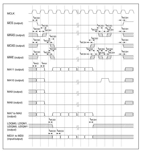
Figure 7.10 UGM Write Cycle Timing
