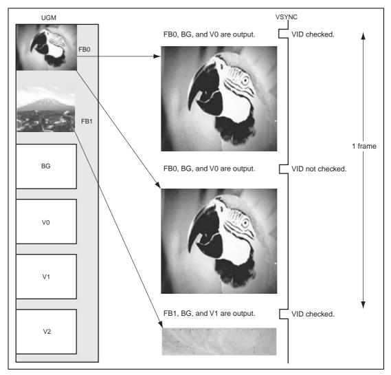
Figure 3.33 Interlace Mode Display Output
