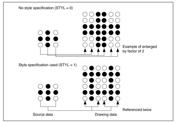
Figure 3.44 Example of Source Style Specification
