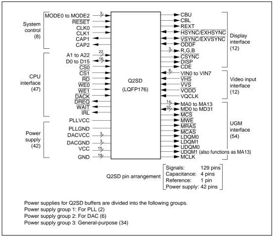
Figure 2.1 Pin Configuration
