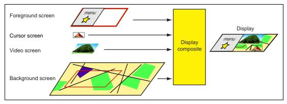
Figure 1.7 Display Composite Function
