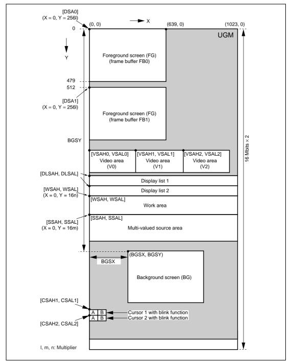
Figure 3.12 Sample Memory Map (Corresponding to  $640 \times 480$  Screen Size, with 16 Bits/Pixel )
