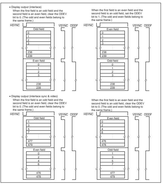
Figure 3.30 Display by Interlace Sync Method
