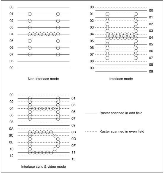
Figure 3.29 Examples of Raster Scan Control Display
