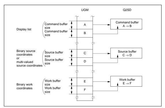
Figure 3.50 Updating of Q2SD's Internal Buffers
