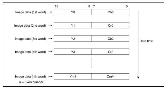
Figure 3.65 The Flow of YCbCr (4:2:2) Data
