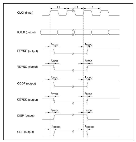
Figure 7.12 Master Mode Display Timing
