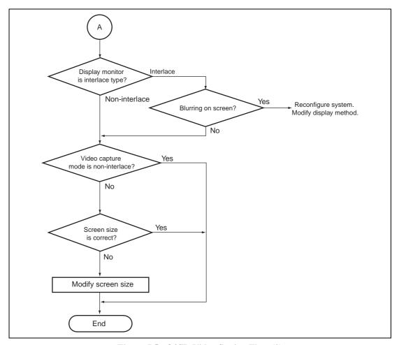
Figure J.5 Q2SD Video Setting Flow (2)
