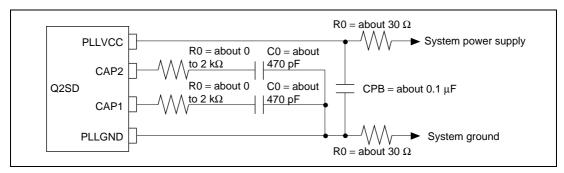
Figure 2.3 Example of Circuit for Connection of Pins CAP1 and CAP2
