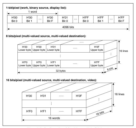
Figure 3.7 Configuration of One Memory Unit (512 Bytes)
