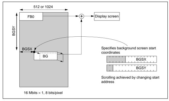
Figure 3.27 Example of Background Screen Simple Scroll (WRAP = 0)
