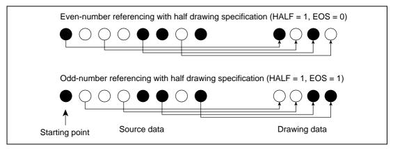
Figure 3.46 Examples of Even/Odd Select Specifications
