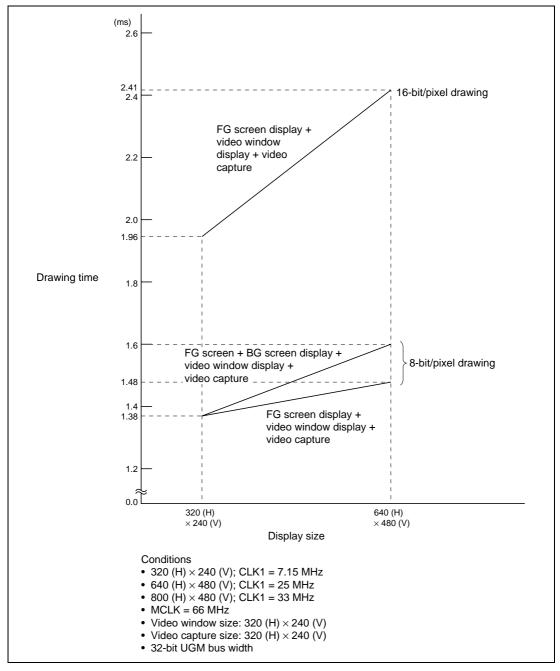
Figure I.3 POLYGON4C Drawing Performance when FST = 0 (Drawing Range: 320 (H)  $\times$  240 (V))
