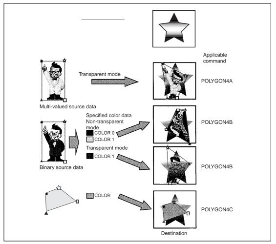
Figure 3.39 Example of POLYGON4 Transfer Data Combinations
