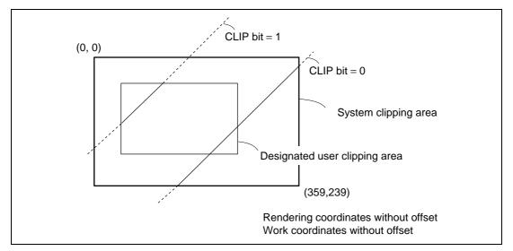
Figure 3.45 Example of Clipping Specification
