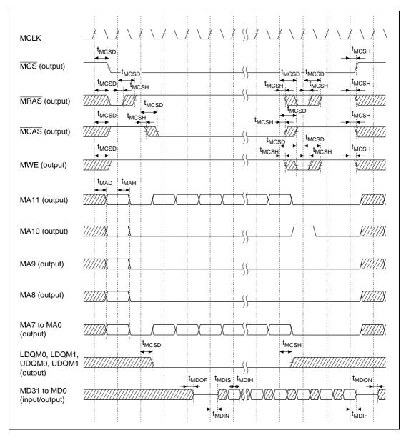
Figure 7.9 UGM Read Cycle Timing
