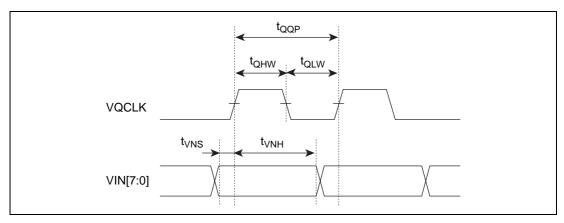
Figure 7.14 (1) Video Interface Timing
