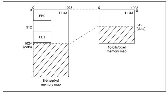
Figure 3.13 Relationship between 8-Bits/Pixel and 16-Bits/Pixel Memory Maps
