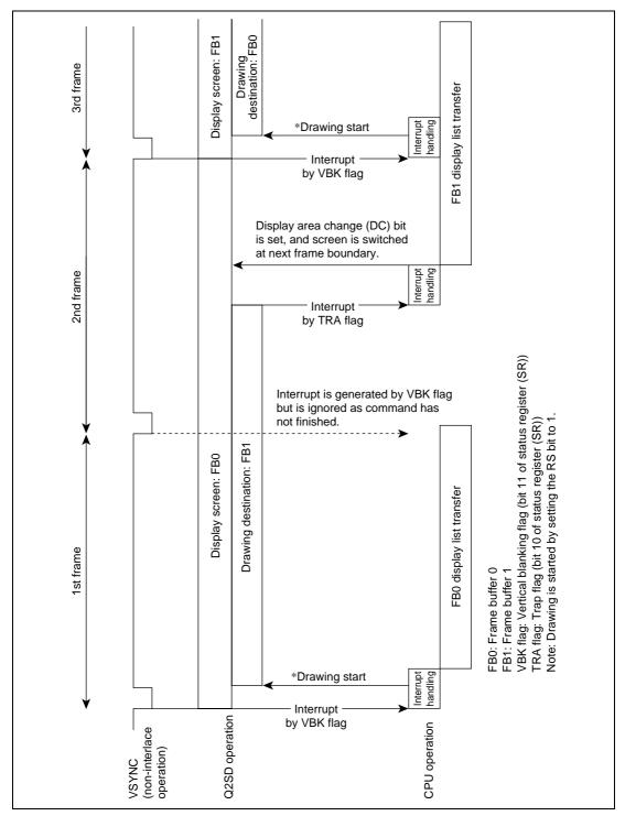
Figure 3.23 Operation in Manual Display Change Mode
