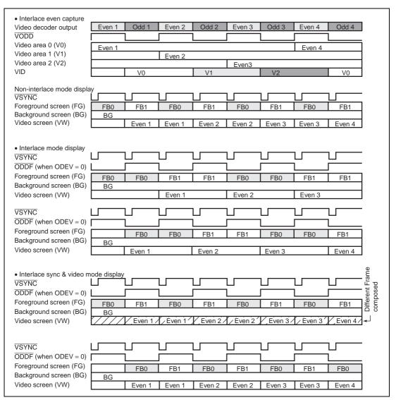
Figure 3.73 The Display of Data Captured in the Interlace Even-Only Mode
