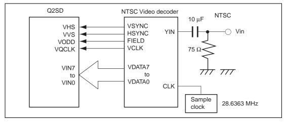
Figure 2.6 Example of Connection of Video Input Pins
