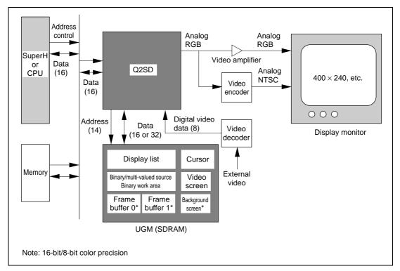
Figure 1.1 Sample System Configuration
