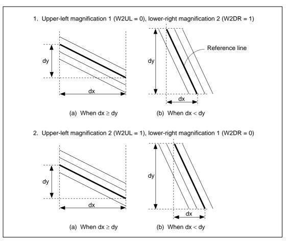
Figure 3.47 Examples of Bold Line Drawing
