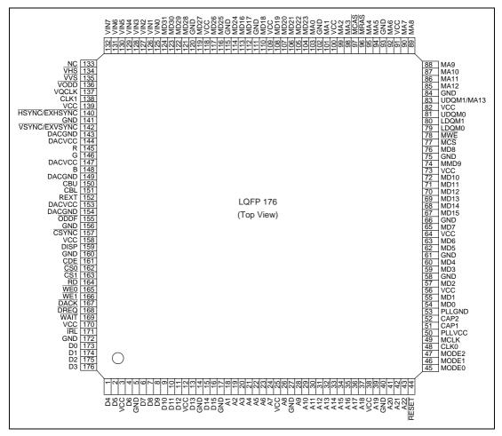
Figure 2.2 Pin Arrangement
