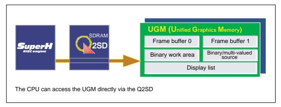
Figure 1.3 Unified System Bus Interface
