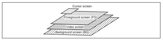
Figure 3.26 Configuration of the Display Screen for Q2SD
