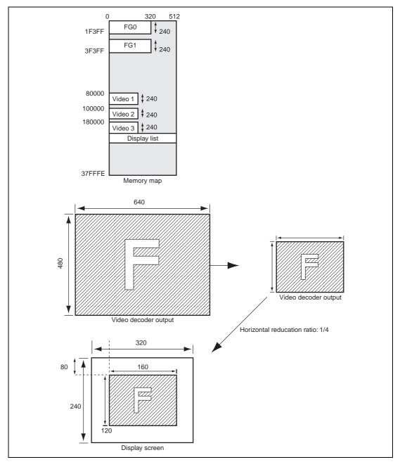
Figure J.2 Interlace Composite Capture (Horizontal and Vertical Reduction Ratios = 1/4)
