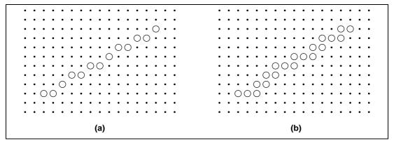
Figure C.1 Two Representations of a Straight Line on a Raster Display
