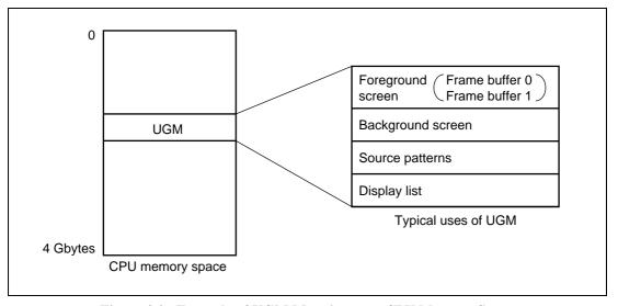
Figure 3.2 Example of UGM Mapping onto CPU Memory Space
