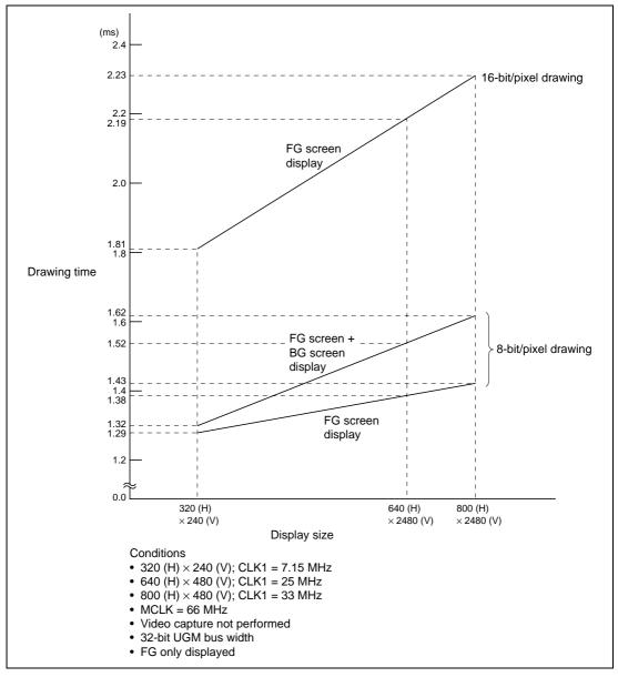
Figure I.1 POLYGON4C Drawing Performance when FST = 0 (Drawing Range:  $320 \text{ (H)} \times 240 \text{ (V)}$ )
