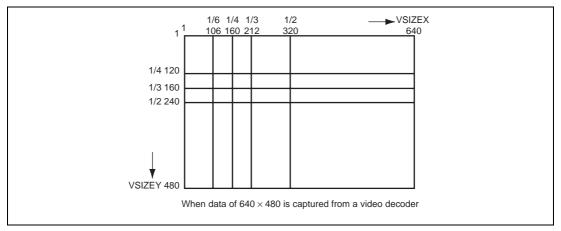
Figure 3.61 Reducing the Size of the Captured Image
