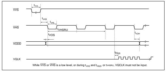
Figure 7.14 (2) Video Interface Timing
