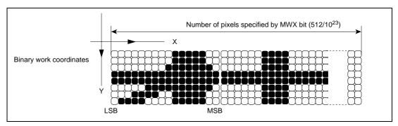
Figure 3.42 Binary Work Data Configuration
