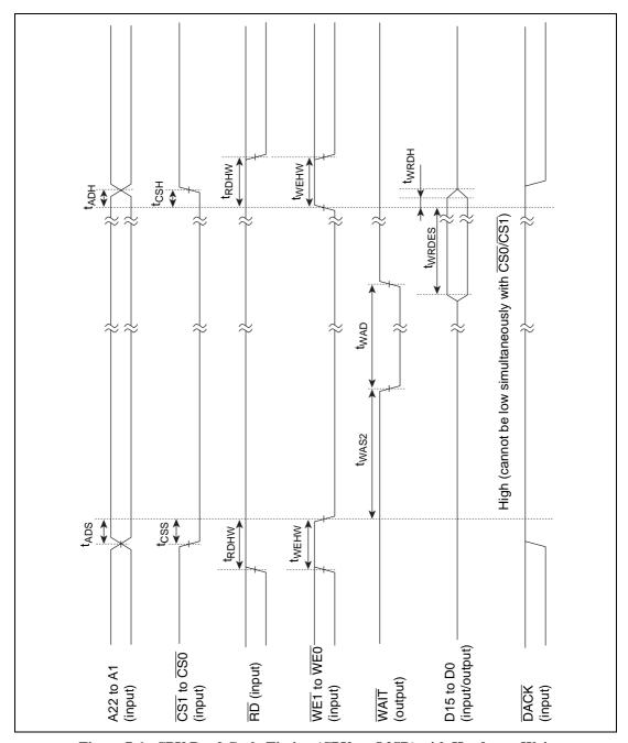
Figure 7.6 CPU Read Cycle Timing (CPU  $\rightarrow$  Q2SD) with Hardware Wait
