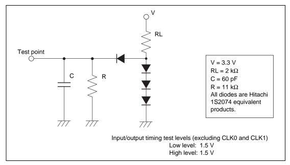
Figure 7.2 Test Load Circuit
