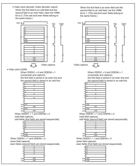
Figure 3.60 Interlace Video Input Field Handling Specification
