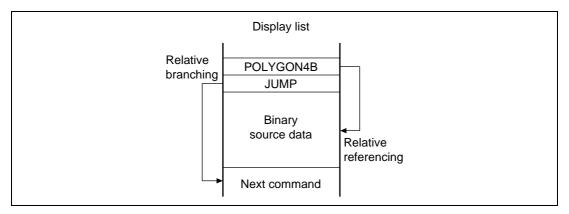
Figure H.2 Example of Referencing and Branching
