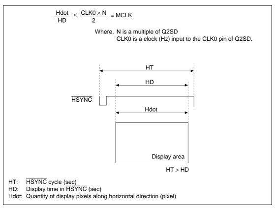
Figure G.1 Example of Display Timing
