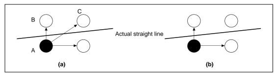
Figure C.3 Drawing Dot Determination Process in (a) 8-Point Drawing and (b) 4-Point Drawing
