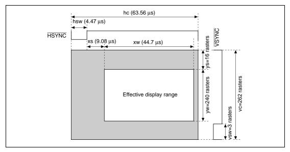
$Figure \ G.2 \quad Example \ of \ Display \ Timing \ under \ Non-interlace \ Mode$
