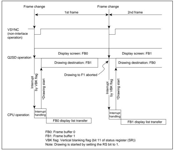
Figure 3.21 Operation in Auto Display Change Mode
