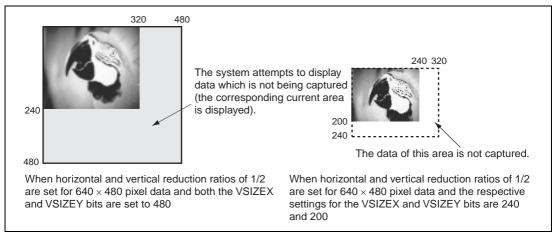
Figure 3.62 Incorrect Settings for the Reduction Ratios
