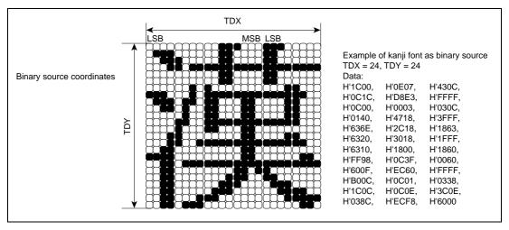
Figure 3.41 Example of Kanji Font as Binary Source (TDX = 24, TDY = 24)
