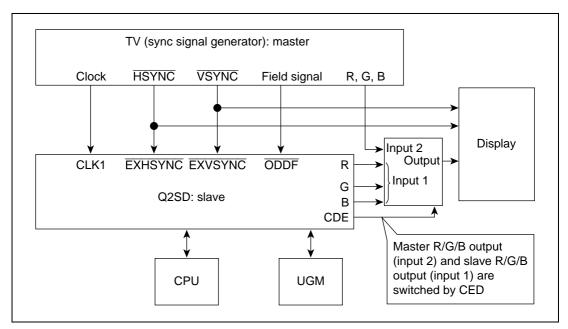
Figure 3.35 Signal Flow in TV Sync Mode
