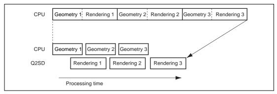
Figure 1.6 Pipeline Graphics Processing
