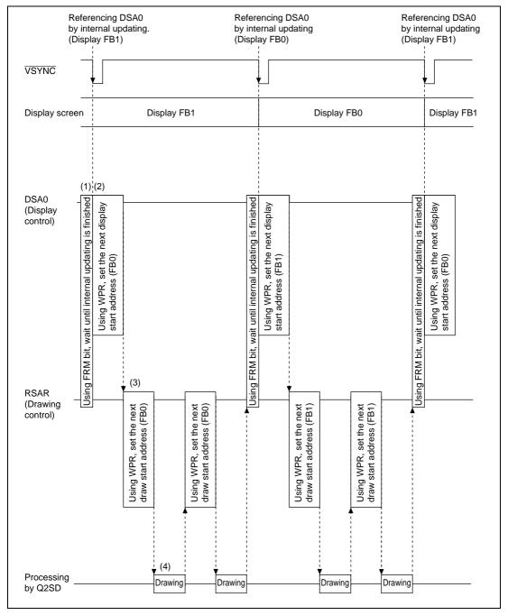
Figure H.1 Display/Drawing Control Timing Chart (DBF = 0)
