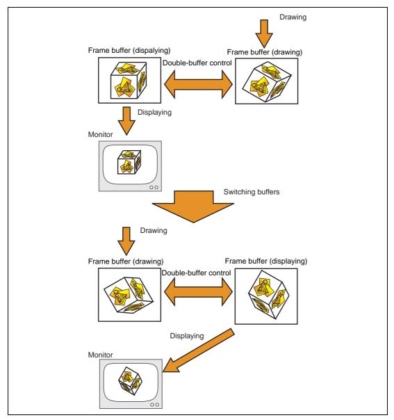
Figure 1.4 Double-Buffering Architecture
