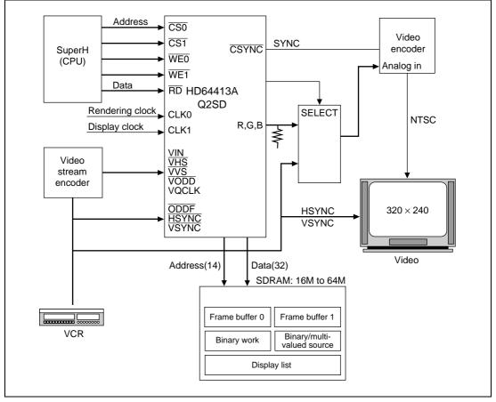
Figure F.1 Example of System Configuration Overview
