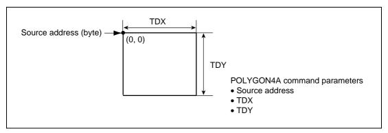
Figure 3.18 Multi-Valued Source Coordinates with LNi = 1 Specified (Linear Address)
