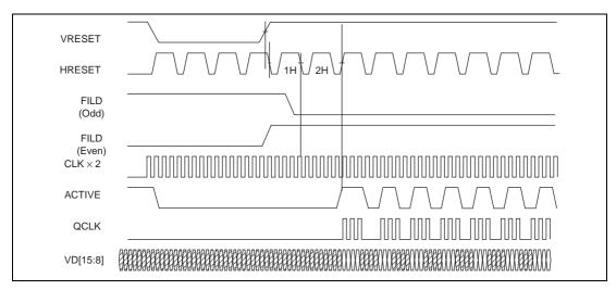
Figure J.8 Example of Interlaced Data Output Timing for Decoder
