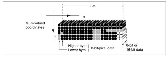
Figure 3.40 Multi-Valued Source Data Configuration
