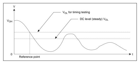
Figure 7.1 Basis of  $V_{\text{OL}}$  Timing Testing
