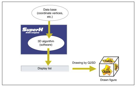
Figure 1.9 Data Flow when Using a 3D Algorithm
