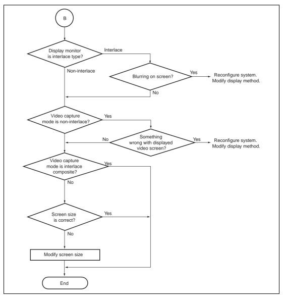
Figure J.6 Q2SD Video Setting Flow (3)
