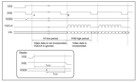
Figure 6.2 Video Interface Timing
