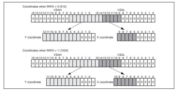
Figure 3.63 Setting up the Capture Area
