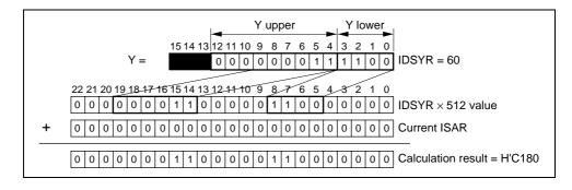
Example: Method of calculating second ISAR, with memory width of 1024 (from figure 3.9)
