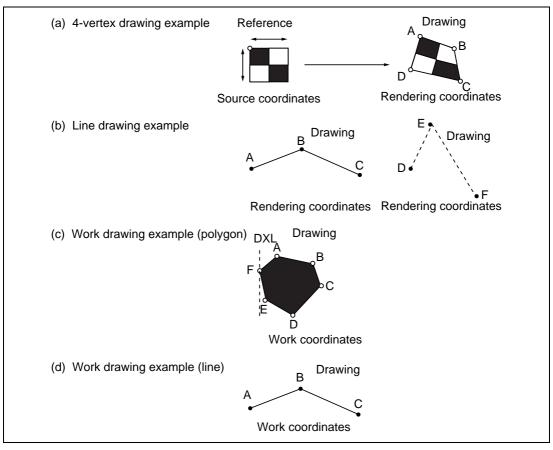
Figure 3.38 Drawing Functions
