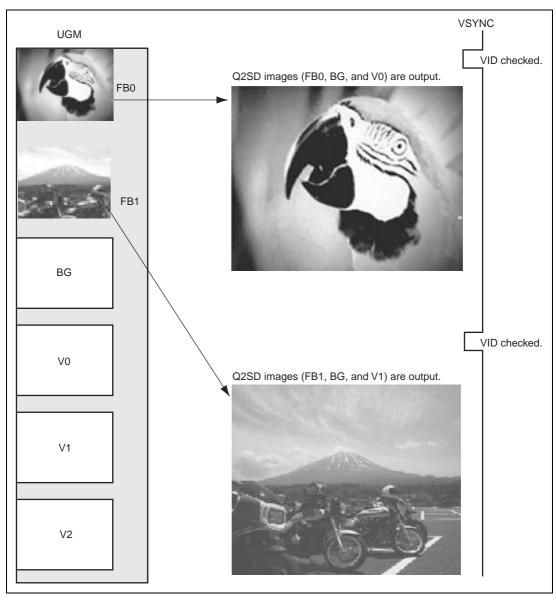
Figure 3.32 Non-Interlace Mode Display Output
