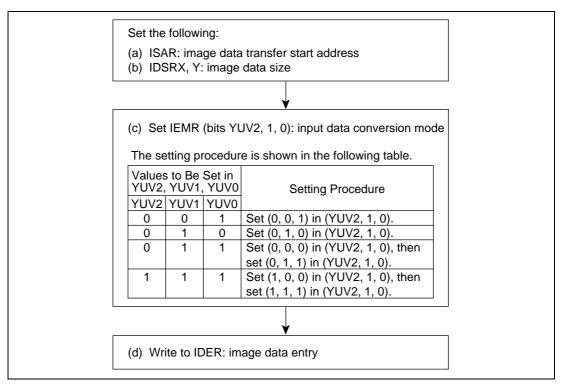
Figure 3.5 Register Setting Procedure for ΔYUV/YUV-to-RGB Conversion
