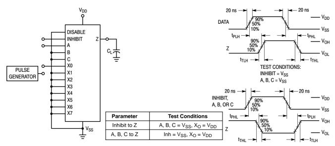
Figure 2. AC Test Circuit and Waveforms
