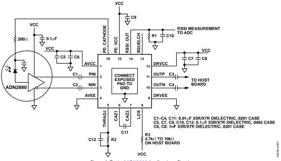
Figure 8. Typical ADN2890 Applications Circuit
