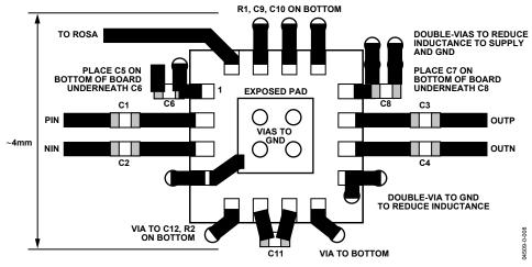
Figure 9. Recommended ADN2890 PCB Layout
