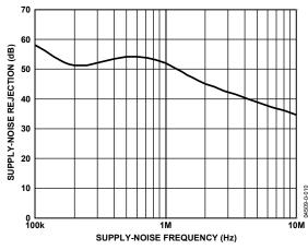
Figure 5. Typical PSRR vs. Supply-Noise Frequency
