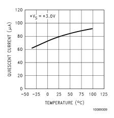
**Typical Performance Characteristics** To generate these curves the LM62 was mounted to a printed circuit board as shown in *Figure 2*. (Continued)
