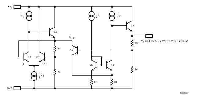
FIGURE 6. Simplified Schematic
