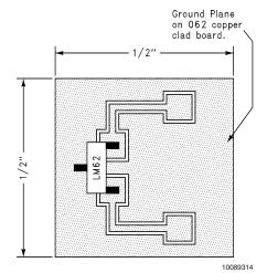
Printed Circuit Board Used for Heat Sink to Generate All Curves. 1/2" Square Printed Circuit Board with 2 oz. Copper Foil or Similar.
