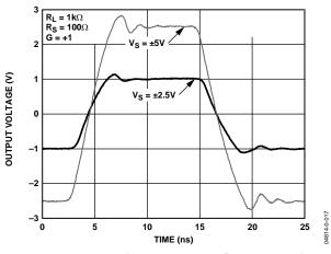
Figure 39. Large Signal Transient Response for Various Supplies
