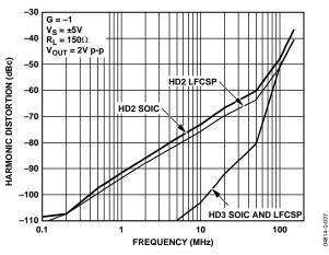
Figure 21. Harmonic Distortion vs. Frequency for Various Packages
