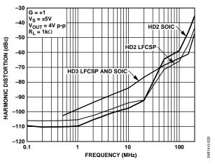
Figure 18. Harmonic Distortion vs. Frequency for Various Packages
