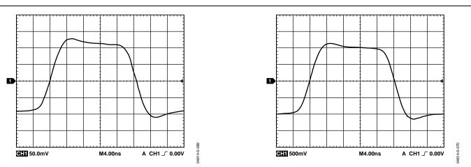
Figure 71. Small Signal Transient Response of 90 MHz LPF
