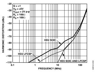
Figure 19. Harmonic Distortion vs. Frequency for Various Packages
