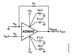
Figure 61. Noninverting Configuration
