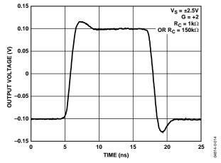
Figure 36. Small Signal Transient Response for Various Loads
