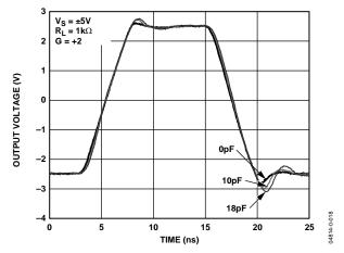
Figure 40. Large Signal Transient Response with Capacitive Load
