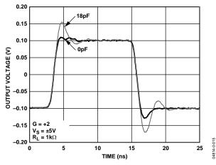
Figure 37. Small Signal Transient Response with Capacitive Load
