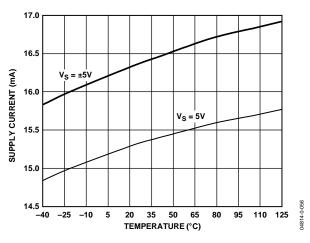
Figure 57. Supply Current vs. Temperature for Various Supplies
