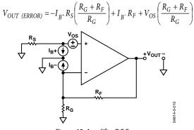
Figure 65. Amplifier DC Errors
