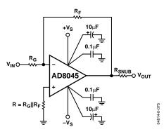
Figure 62. Inverting Configuration
