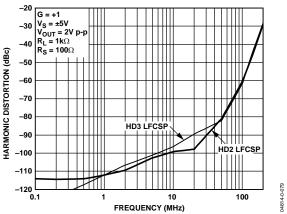
Figure 3. Harmonic Distortion vs. Frequency for Various Packages
