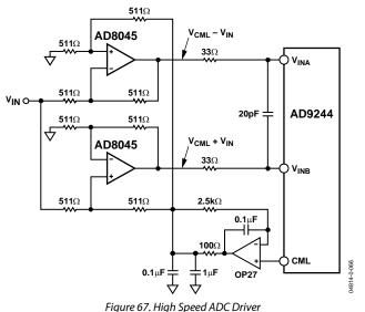
The outputs of the AD8045 devices are centered about the 2.5 V common-mode range of the AD9244. The common-mode reference voltage from the AD9244 is buffered and filtered via the OP27 and fed to the noninverting resistor network used in the level shifting circuit.
