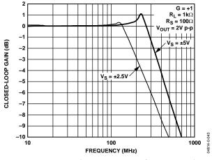
Figure 13. Large Signal Frequency Response for Various Supplies
