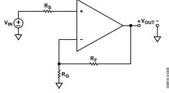
Figure 64. Noninverting Configuration
