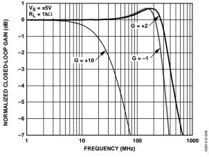
Figure 7. Small Signal Frequency Response for Various Gains
