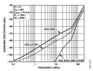
Figure 22. Harmonic Distortion vs. Frequency for Various Packages
