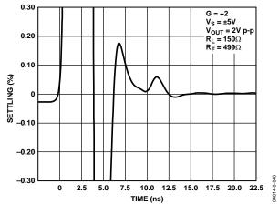
Figure 60. Short Term 0.1% Settling Time
