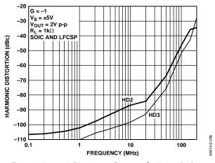
Figure 20. Harmonic Distortion vs. Frequency for Various Packages
