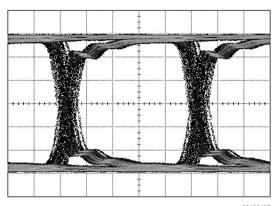
Figure 5. Equalized Signal (40 in FR4, 2.5 Gbps, PRBS7, 0x07 Setting)
