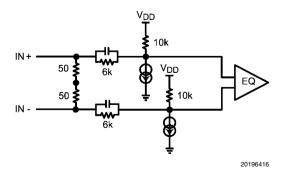
FIGURE 4. Simplified Receiver Input Termination Circuit
