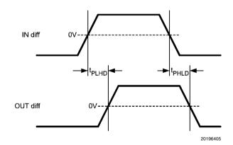
FIGURE 3. Propagation Delay Timing Diagram
