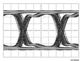
Figure 6. Equalized Signal (40 in FR4, 5 Gbps, PRBS7, 0x07 Setting)
