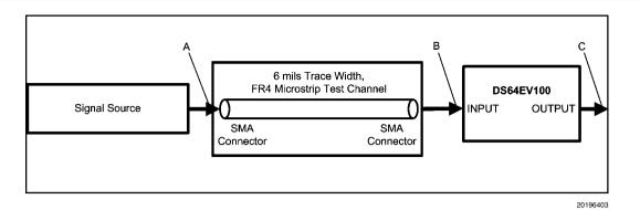
FIGURE 1. Test Setup Diagram
