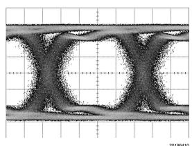
Figure 8. Equalized Signal (40 in FR4, 6.4 Gbps, PRBS31, 0x06 Setting)
