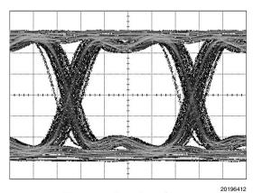
Figure 10. Equalized Signal (10m 24 AWG Twin-AX Cable, 6.4 Gbps, PRBS7, 0x06 Setting)
