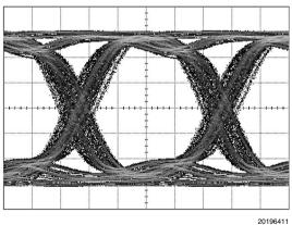
Figure 9. Equalized Signal (30 in FR4, 10 Gbps, PRBS7, 0x06 Setting)
