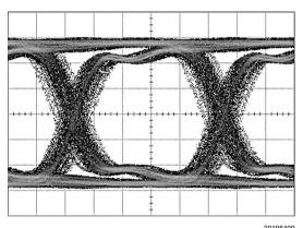
Figure 7. Equalized Signal (40 in FR4, 6.4 Gbps, PRBS7, 0x06 Setting)
