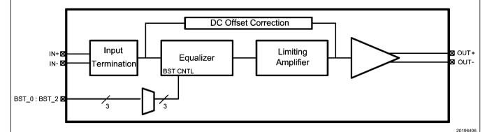
FIGURE 5. Simplified Block Diagram
