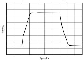
LARGE SIGNAL STEP RESPONSE (G = -1V/V, R<sub>L</sub> = 10k $\Omega$ , C<sub>L</sub> = 15pF)
