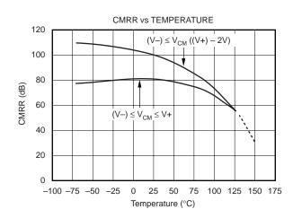
At  $T_A$  = +25°C,  $V_S$  =  $\pm 6V$ , and  $R_L$  = 10k $\Omega$ , unless otherwise noted.
