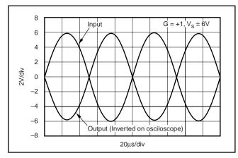
FIGURE 1. Rail-to-Rail Input and Output.
