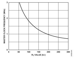
Figure 4. Master Clock Frequency vs.  $R_T$
