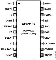
Figure 3. Pin Configuration
