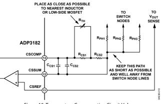
Figure 10. Temperature Compensation Circuit Values
