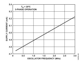
Figure 5. Supply Current vs. Oscillator Frequency
