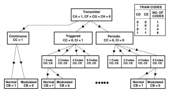
Figure 5–6. Transmitter Configurations
