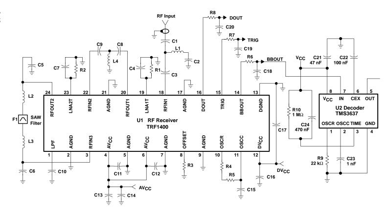
Figure 6–8. TRF1400 RF Receiver and TMS3637 Decoder Circuit
