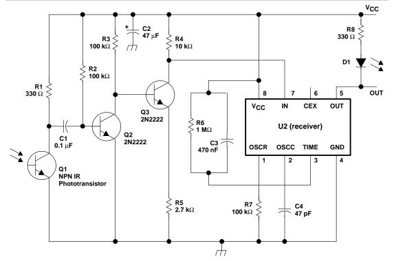
Figure 6–5. Infrared Receiver
