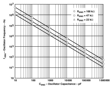
Figure 4–2. Oscillator Frequency Versus Oscillator Capacitance
