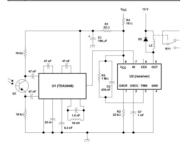
Figure 6–6. Infrared Modulated Receiver
