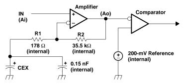
Figure 5–3. Amplifier/Comparator Schematic
