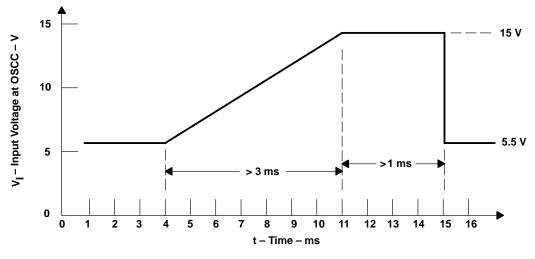
Figure 4–3. High-Voltage Programming Pulse
