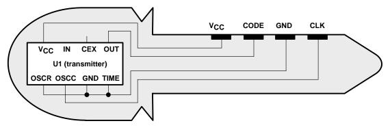
Figure 6–3. Four-Wire Direct Connection Key
