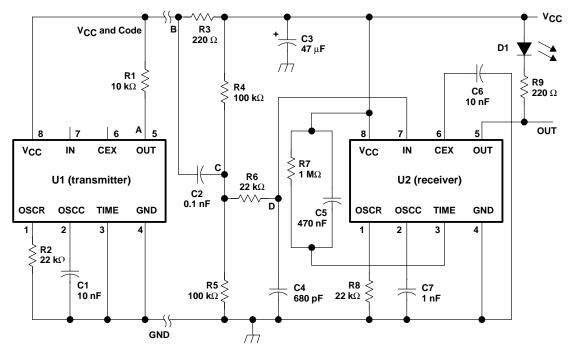
Figure 6–1. Two-Wire Direct Connection
