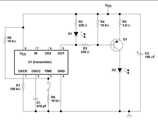
Figure 6–4. Infrared Transmitter
