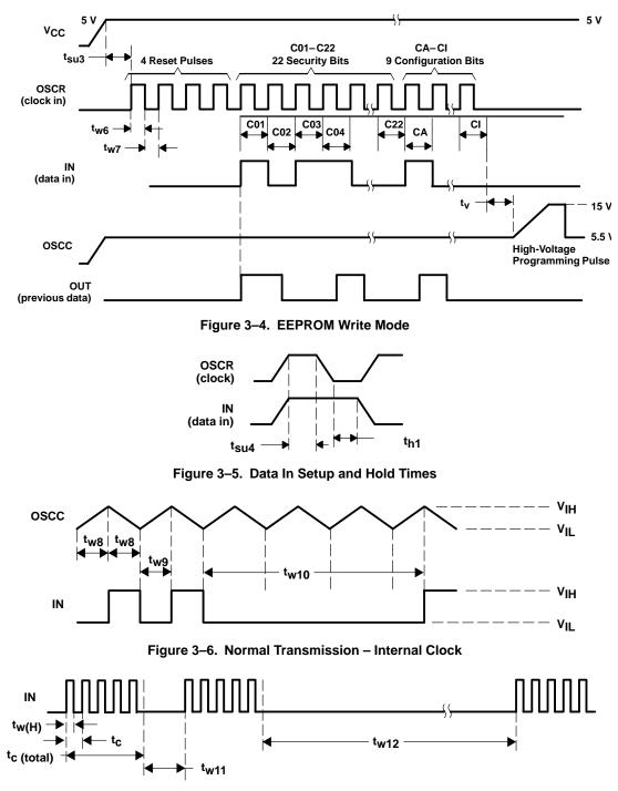
Figure 3–7. Modulated Transmission – Internal Clock
