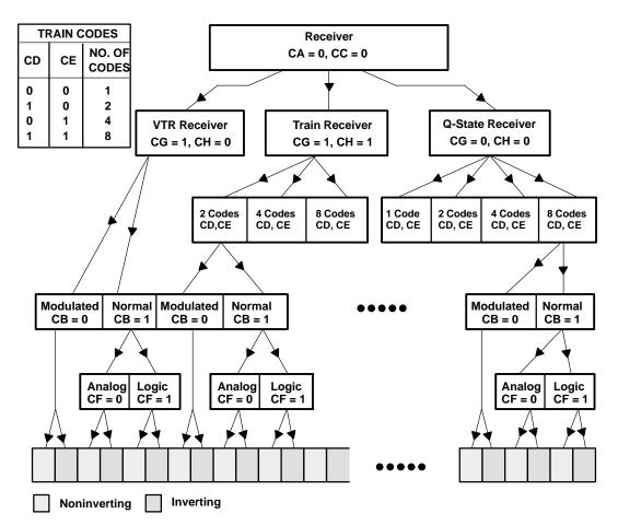
Figure 5–7. Receiver Configurations
