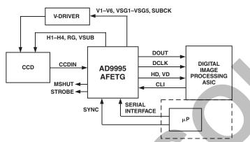
Figure 1. Typical System Block Diagram, Master Mode
