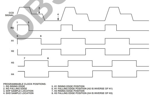
Figure 5. High Speed Clock Programmable Locations
