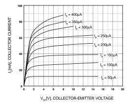
Figure 1. Static Characteristic
