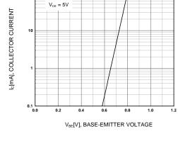
Figure 2. Transfer Characteristic
