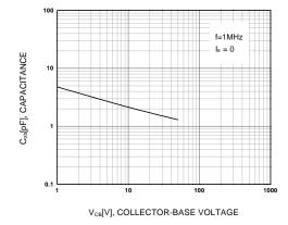
Figure 5. Output Capacitance
