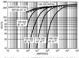
FIGURE 2. V-I CHARACTERISTIC RESPONSE TO NEUTRON IRRADIATION FOR MOV AND ZENER DIODE DEVICES
