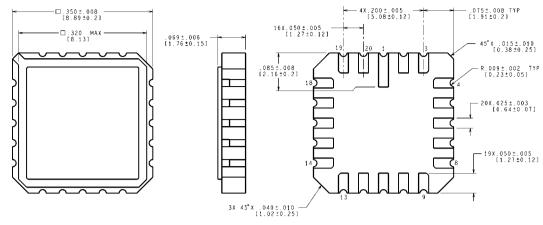
CONTROLLING DIMENSION IS INCH VALUES IN [] ARE MILLIMETERS
