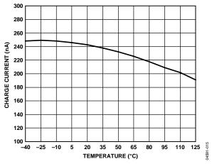
Figure 15. CEXT Charge Current vs. Temperature
