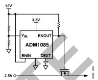
Figure 31. Sequencing with a FET Switch
