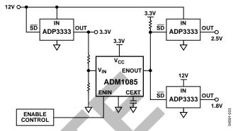
Figure 28. Enabling a Pair of Regulators from a Single ADM1085
