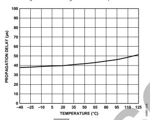
Figure 16.  $V_{\mathbb{N}}$  to ENOUT/ $\overline{\text{ENOUT}}$  Propagation Delay (CEXT Floating) vs. Temperature
