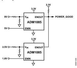
Figure 30. Quad-Supply Power Good Indicator
