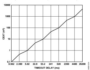
Figure 14. CEXT Capacitance vs. Timeout Delay
