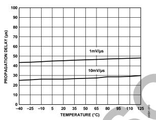
Figure 10. Vcc Falling Propagation Delay vs. Temperature
