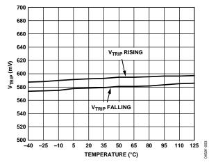
Figure 3. V<sub>IN</sub> Threshold vs. Temperature
