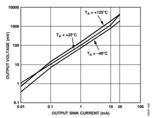
Figure 8. Output Voltage vs. Output Sink Current
