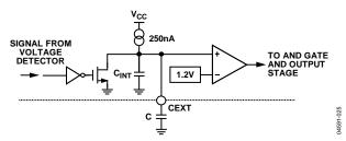
Figure 20. Capacitor-Adjustable Delay Circuit
