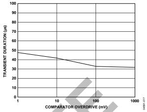
Figure 17. Maximum V<sub>IN</sub> Transient Duration vs. Comparator Overdrive
