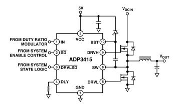
Figure 1. Typical Application Circuit
