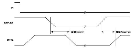
Figure 3. DRVLSD Propagation Delay
