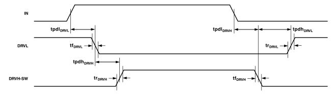
Figure 4. Switching Timing Diagram (Propagation Delay Referenced to 50%, Rise and Fall Time to 10% and 90% Points)
