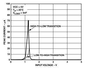
TPC 3. Input Voltage vs. Input Current
