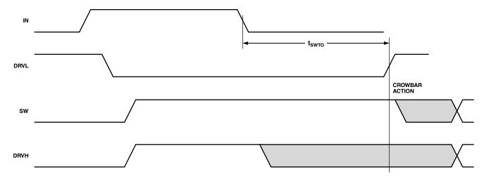
Figure 5. Switching Waveforms–SW Node Failure Mode–DRVL Timeout
