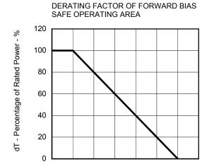
TOTAL POWER DISSIPATION vs. CASE TEMPERATURE
