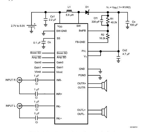
FIGURE 1. Typical LM48520 Audio Amplifier Application Circuit
