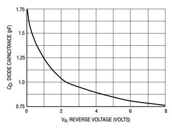
Figure 3. Diode Capacitance
