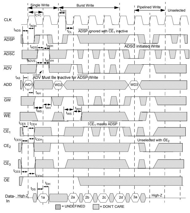
**Notes:** 14. WE is the combination of  $\overline{BWE}$ ,  $\overline{BW}_{[3:0]}$  and  $\overline{GW}$  to define a Write cycle (see Write Cycle Descriptions table). 15. WDx stands for Write Data to Address X.
