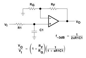
Figure 44. Single-Pole Low-Pass Filter
