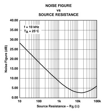
Figure 41. Noise Figure vs Source Resistance
