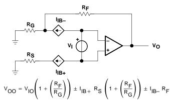
Figure 43. Output Offset Voltage Model
