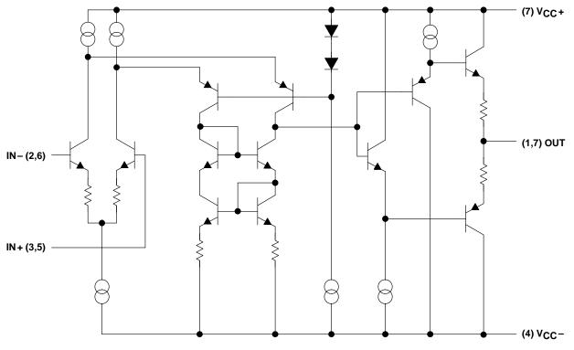
Figure 39. THS6072 Simplified Schematic
