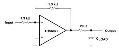
Figure 42. Driving a Capacitive Load
