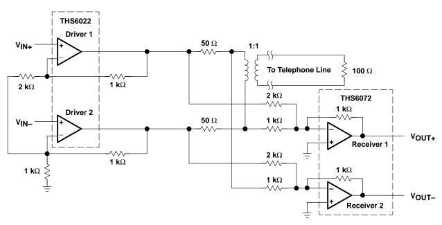
Figure 38. Typical ADSL Remote Terminal Application
