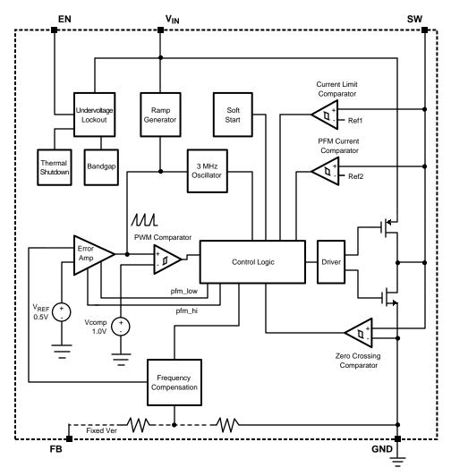
Figure 4. Simplified Functional Diagram
