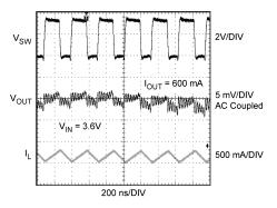
Figure 46. Typical PWM Operation
