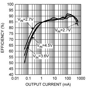
Figure 3. Efficiency vs. Output Current  $(V_{OUT} = 1.8V)$
