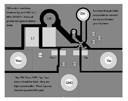
Figure 49. Board Layout Design Rules for the LM3677
