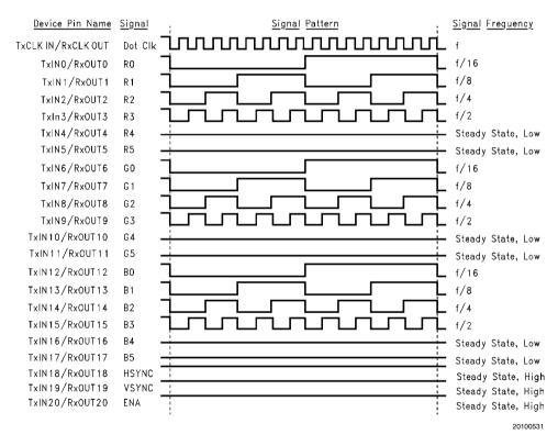
FIGURE 2. "16 Grayscale" Test Pattern - DS90C365A (Notes 8, 9, 10)
