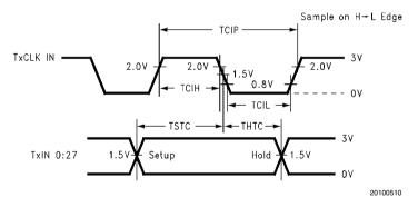
FIGURE 6. DS90C365A (Transmitter) Setup/Hold and High/Low Times with R\_FB pin = GND (Falling Edge Strobe)
