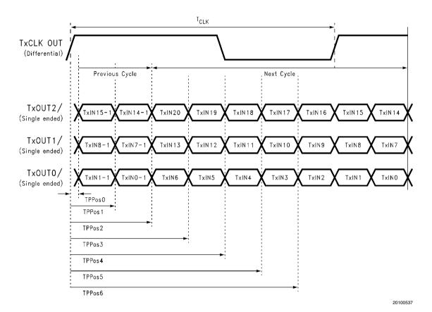
FIGURE 12. Transmitter LVDS Output Pulse Position Measurement - DS90C365A
