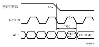
FIGURE 11. Transmitter Power Down Delay
