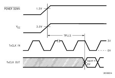
FIGURE 9. DS90C365A (Transmitter) Phase Lock Loop Set Time
