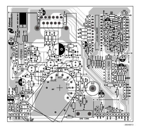
FIGURE 16. LM126X/LM242X/LM248X Demonstration Board Layout
