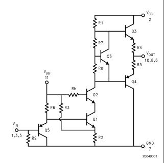
FIGURE 2. Simplified Schematic Diagram (One Channel)
