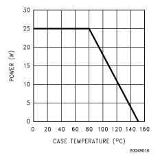
FIGURE 11. Power Derating Curve
