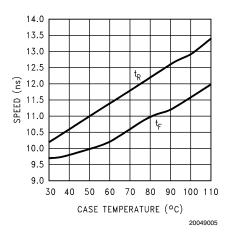
FIGURE 9. Speed vs Case Temperature
