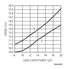
FIGURE 7. Speed vs Load Capacitance
