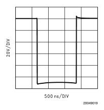
FIGURE 12. Cathode Pulse Response
