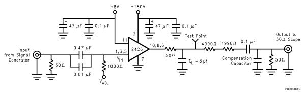
Note: 8pF load includes parasitic capacitance.
