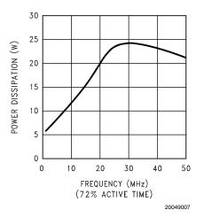
FIGURE 10. Power Dissipation vs Frequency
