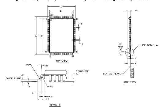
Figure 8. 100-pin TQFP (14 × 20 × 1.4 mm) A100RA Package Outline, 51-85050
