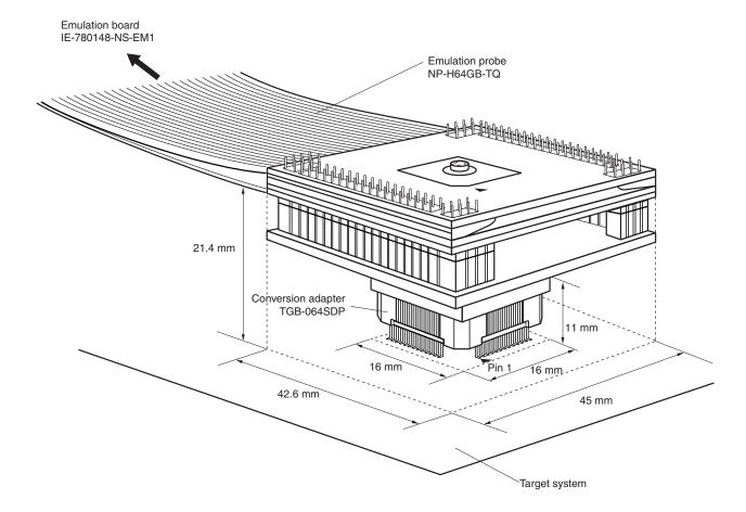
Figure B-3. Connection Conditions of Target System (When Using NP-H64GB-TQ)
