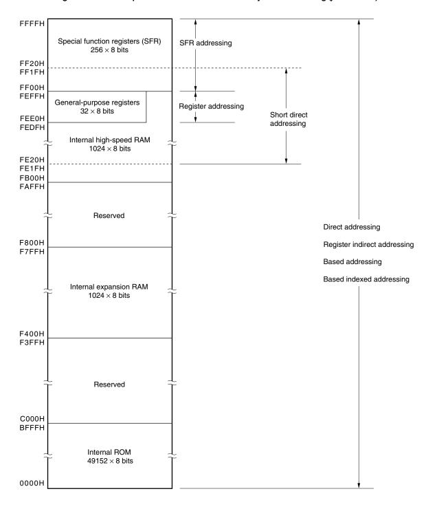
Figure 3-14. Correspondence Between Data Memory and Addressing (µPD780136)
