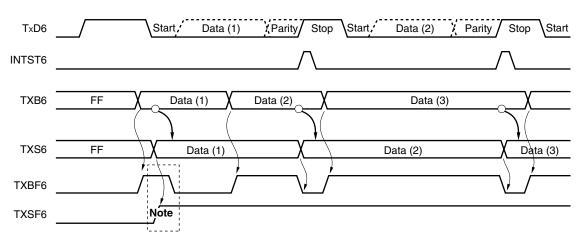
Figure 14-17. Timing of Starting Continuous Transmission
