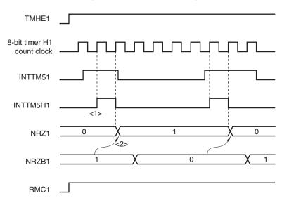
Figure 8-13. Transfer Timing
