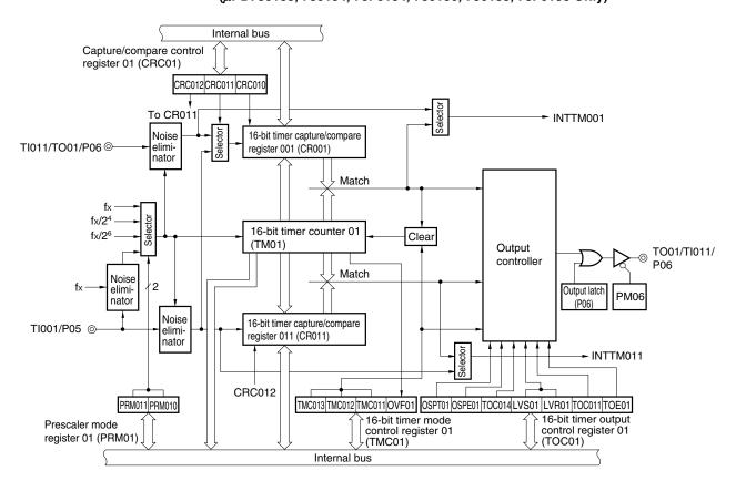
Figure 6-2. Block Diagram of 16-Bit Timer/Event Counter 01 (μPD780133, 780134, 78F0134, 780136, 780138, 78F0138 Only)
