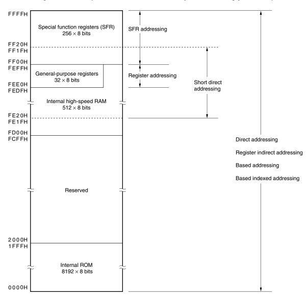
Figure 3-9. Correspondence Between Data Memory and Addressing (μPD780131)
