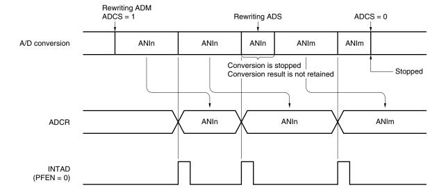
Figure 12-11. A/D Conversion Operation
