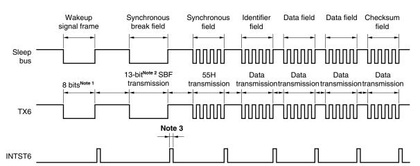
Figure 14-1. LIN Transmission Operation
