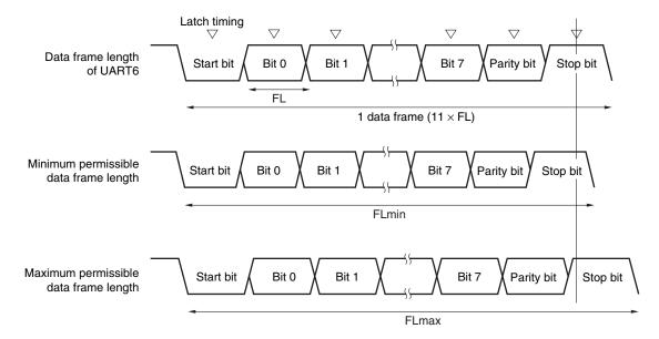
Figure 14-26. Permissible Baud Rate Range During Reception
