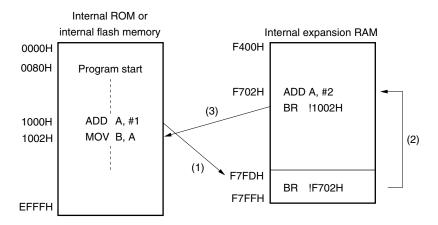
Figure 26-4. ROM Correction Usage Example
