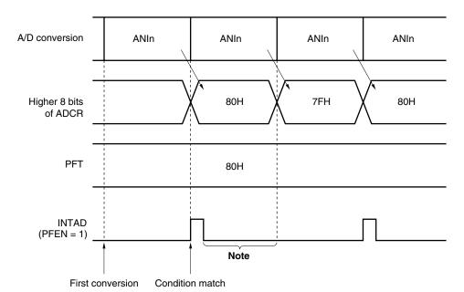
Figure 12-12. Power-Fail Detection (When PFEN = 1 and PFCM = 0)
