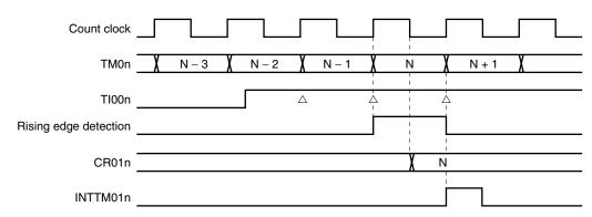
Figure 6-21. CR01n Capture Operation with Rising Edge Specified
