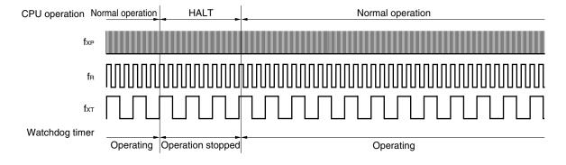
Figure 10-8. Operation in HALT Mode
