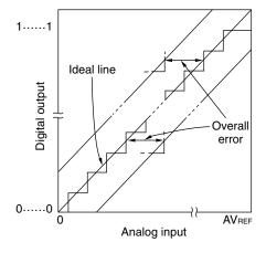
Figure 12-14. Quantization Error
