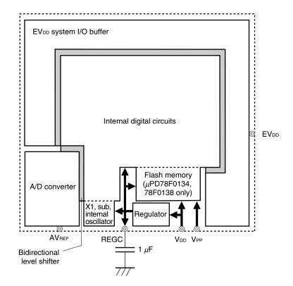
Figure 24-1. Block Diagram of Regulator Periphery
