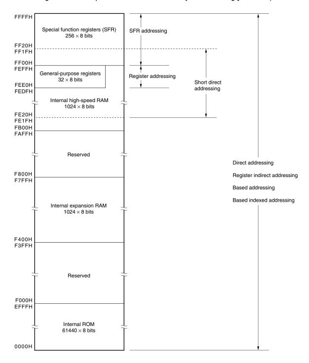
Figure 3-15. Correspondence Between Data Memory and Addressing (µPD780138)
