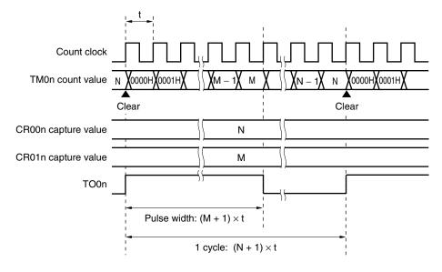
Figure 6-20. PPG Output Operation Timing
