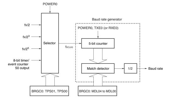
Figure 13-11. Configuration of Baud Rate Generator
