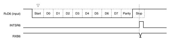
Figure 14-19. Reception Completion Interrupt Request Timing
