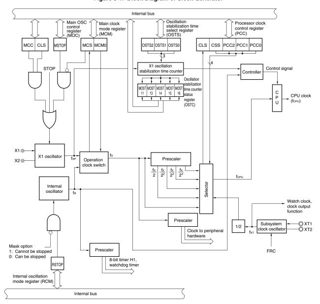
Figure 5-1. Block Diagram of Clock Generator
