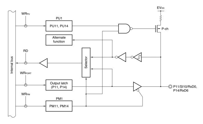
Figure 4-7. Block Diagram of P11 and P14
