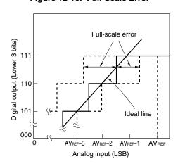
Figure 12-18. Differential Linearity Error
