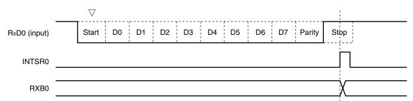
Figure 13-9. Reception Completion Interrupt Request Timing
