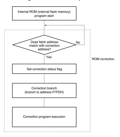
Figure 26-7. ROM Correction Operation
