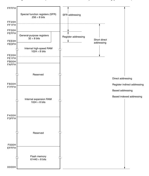
Figure 3-16. Correspondence Between Data Memory and Addressing (µPD78F0138)
