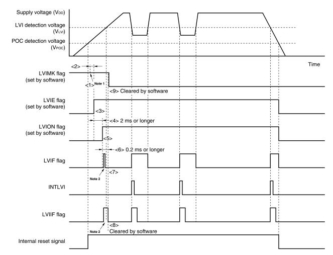
Figure 23-5. Timing of Low-Voltage Detector Interrupt Signal Generation
