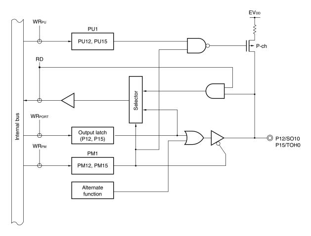
Figure 4-8. Block Diagram of P12 and P15
