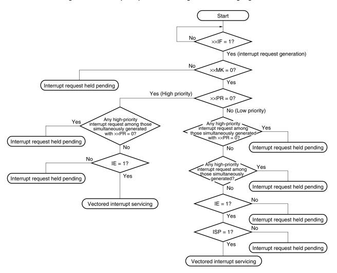
Figure 17-7. Interrupt Request Acknowledgment Processing Algorithm
