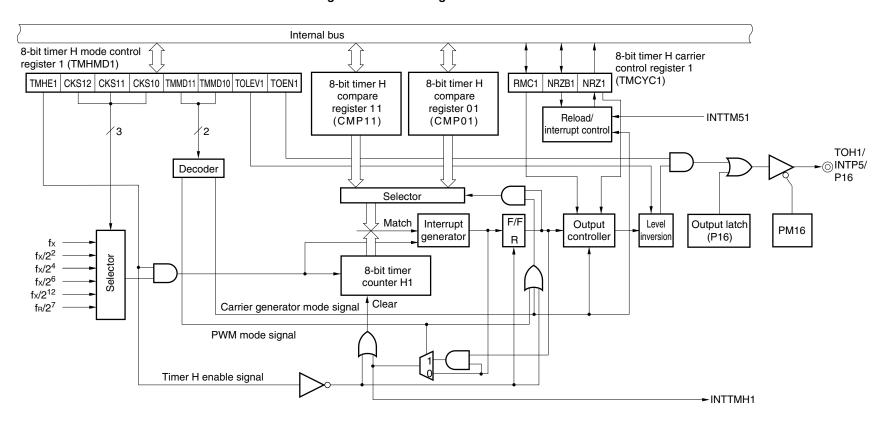
Figure 8-2. Block Diagram of 8-Bit Timer H1
