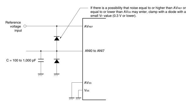
Figure 12-19. Analog Input Pin Connection
