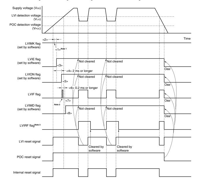
Figure 23-4. Timing of Low-Voltage Detector Internal Reset Signal Generation
