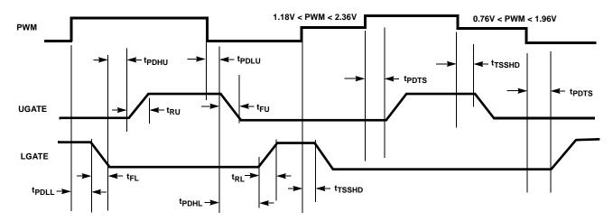
FIGURE 1. TIMING DIAGRAM
