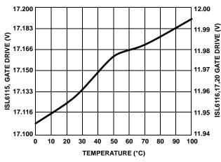
FIGURE 10. GATE DRIVE VOLTAGE, VDD = 12V
