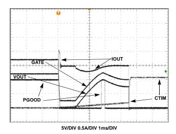
FIGURE 14. ISL6115 'LOW' OVERCURRENT RESPONSE
