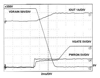
FIGURE 19. +350V LOW SIDE SWITCHING CGATE = 100pF
