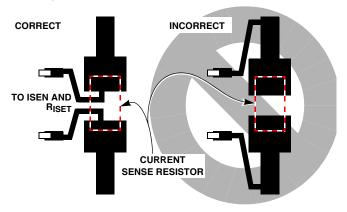
FIGURE 1. SENSE RESISTOR PCB LAYOUT
