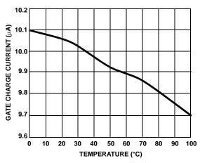
FIGURE 9. GATE CHARGE CURRENT
