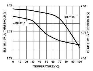
FIGURE 7. ISL6115, ISL6116 UV THRESHOLD
