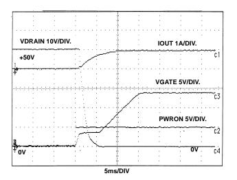
FIGURE 17. +50V LOW SIDE SWITCHING CGATE = 100pF
