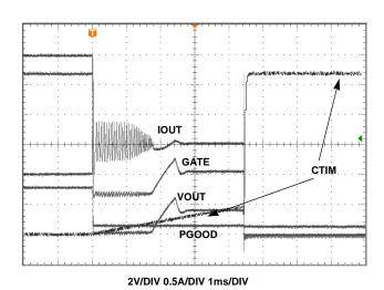
FIGURE 16. ISL6116 'HIGH' OVERCURRENT RESPONSE
