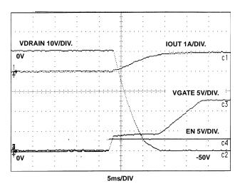
FIGURE 18. -50V LOW SIDE SWITCHING CGATE = 1000pF
