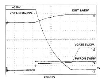
FIGURE 20. +350V LOW SIDE SWITCHING CGATE = 1000pF
