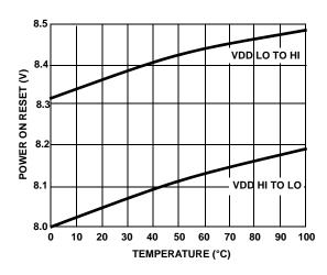
FIGURE 11. POWER ON RESET VOLTAGE THRESHOLD
