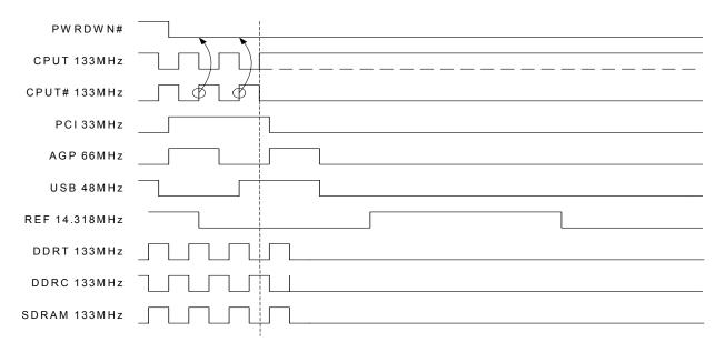
Figure 2. Power-down Assertion Timing Waveform (in P4 mode)
