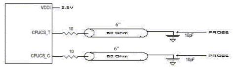
Figure 9. CS Load Termination
