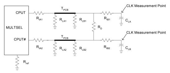
Figure 10. P4 Load Termination
