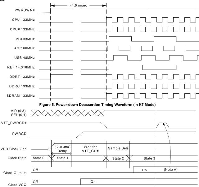
Figure 6. VTT\_PWGD# Timing Diagram (With Advanced PIII Processor SelP4\_K7 = 1) $^{[3]}$
