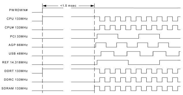
Figure 3. Power-down Deassertion Timing Waveform (in P4 mode)
