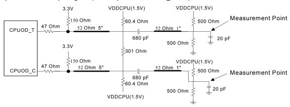
Figure 8. K7 Load Termination
