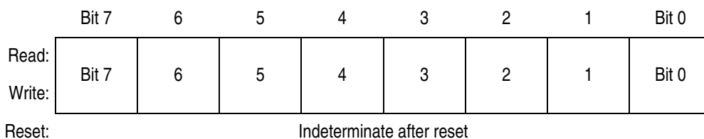
Figure 11-15. TIM Channel 1 Register Low (TCH1L)
