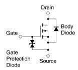
**Remark** The diode connected between the gate and source of the transistor serves as a protector against ESD. When this device actually used, an additional protection circuit is externally required if a voltage exceeding the rated voltage may be applied to this device.
