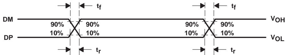
Figure 1. Differential Driver Switching Load
