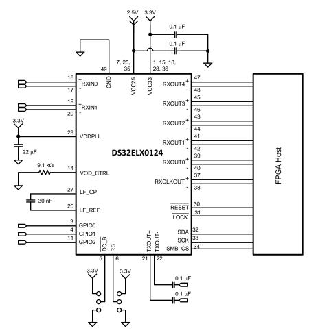
Figure 14. Typical Interface Circuit
