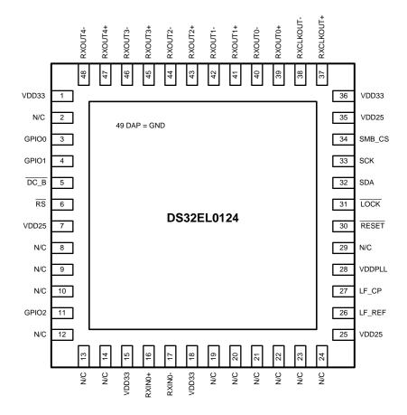
Figure 1. WQFN Package Package Number RHS0048A
