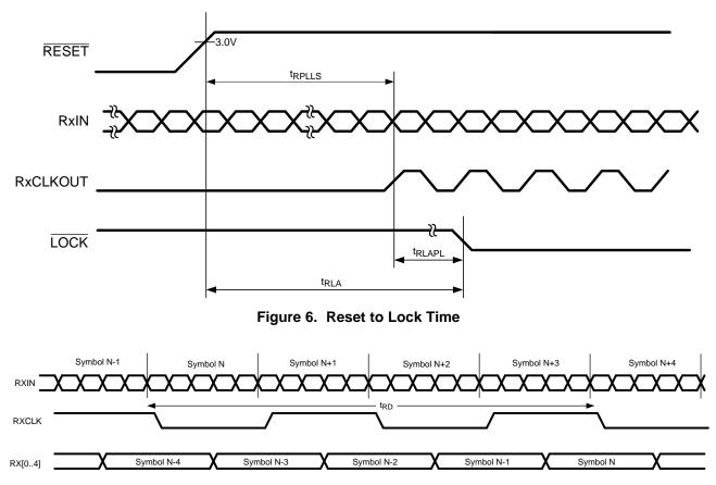
Figure 7. Deserializer Propagation Delay
