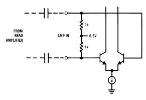
FIGURE 3. Input to Gain Controlled Amplifier
