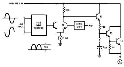
FIGURE 6. Simplified AGC Circuit
