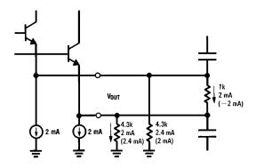
FIGURE 5. Output Stage with 1k Differential Load
