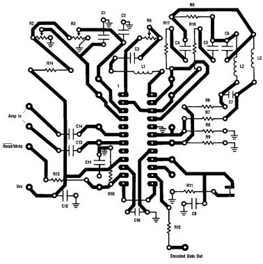
FIGURE 22. DP8464B Component Layout—Top View
